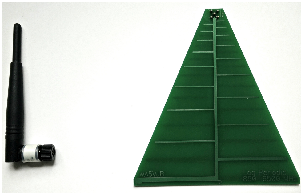
Figure 3.3: Omnidirectional and Directional Antennae
