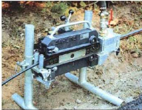
Figure E.3: Blowing a fiber optic cable [21]
