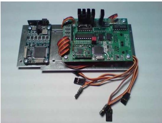
Figure 4.15: The servoboard mounted on the alu-plate together with the IMU.
