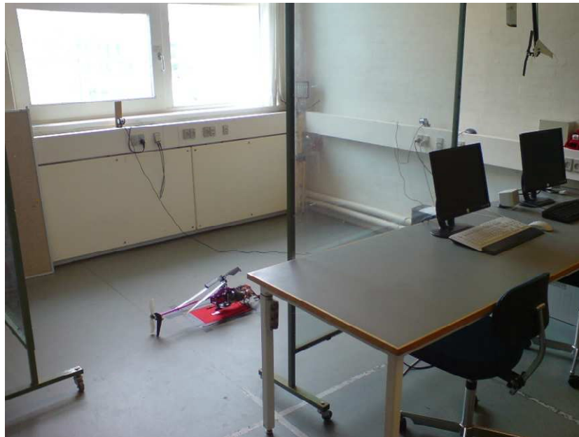
Figure 4.4: The lab where the flight tests take place. The computers controlling the helicopter is seen in the right side. The pilot is placed to the left, such that the helicopter has the rear end towards him. The frontcam is mounted on the wall in front of the helicopter, and the sidecam is mounted on the wall below the window.
