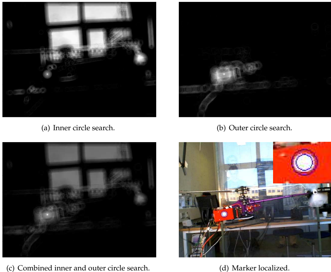
Figure 6.7: The output of the accumulator array of the CHT shown for inner circle search, outer circle search and combined search of the image in Figure 6.5(b) shown in (a), (b) and (c). The resulting estimated marker position is drawn on the image in (d).
