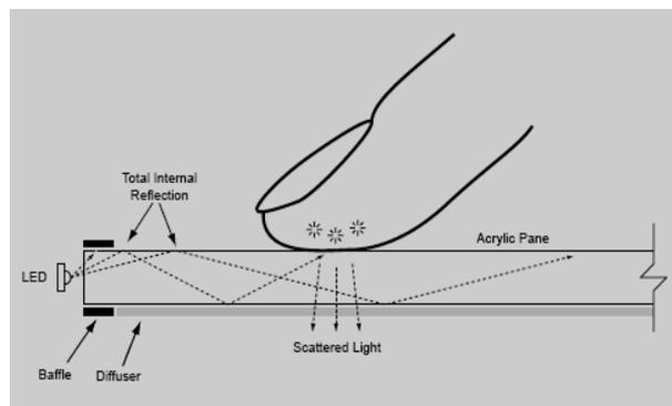
*Fig. 1.1.2: FTIR glass side view [3]*
