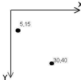
*Fig. 3.1.1: The Java2D coordinate system*
