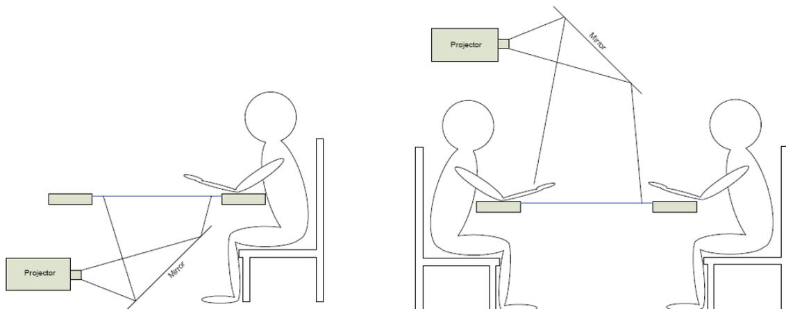
*Fig. 2.1.1: Tabletop, side view, bottom and top projection*
