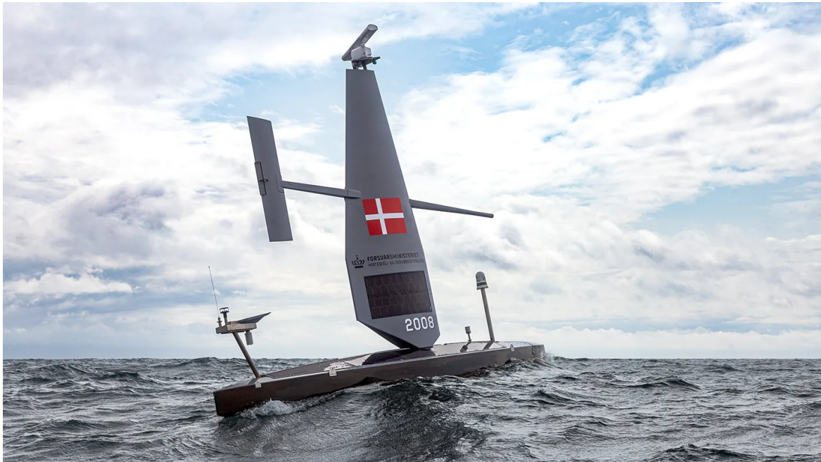
Figure 2.7: Saildrone Voyager USV: A 10-meter autonomous surface vessel utilizing wind and 4 kW electric power for 180-day maritime missions. [81]
