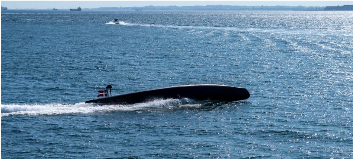
Figure 2.8: Technical specifications of the Copenhagen Orca USV (13 m, 5.5 tons). Features a top speed >40 knots, an 825 kg payload capacity, and an operational range of 500 to 1,400 nm. Mission endurance spans from 3 to 6 weeks depending on configuration [88].
