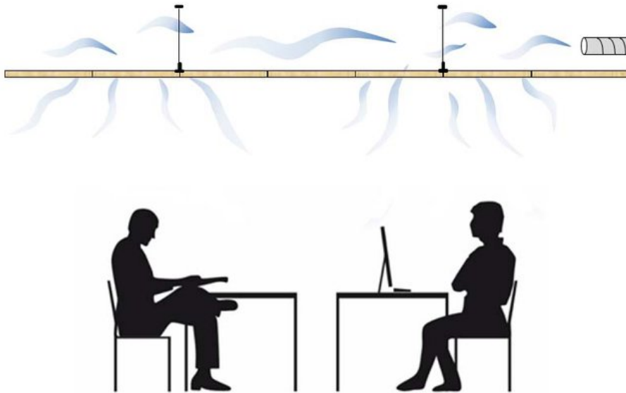
Figure 2.2: Schematic illustration of diffuse ceiling ventilation, showing supply air entering through the ceiling and diffusing into the occupied zone at low velocity. Adapted from Zhang, 2016.
