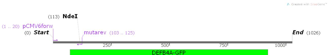
**Figure 2.7.** In the first PCR, pCMV6forw and mutarev primers are used. This creates a product (mut1) with part of the DEFB4A-GFP gene, now with a mutation on the NdeI restriction site. Created with SnapGene software.
