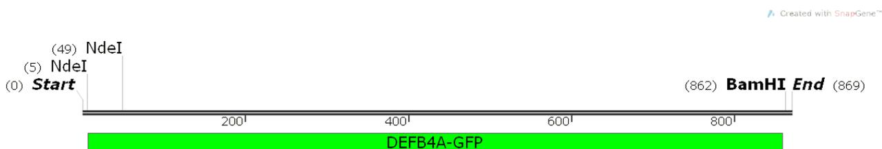
**Figure 2.2.** A second NdeI restriction sequence is found inside the DEFB4A-GFP gene, which makes a normal subcloning procedure inept. Created with SnapGene software.
