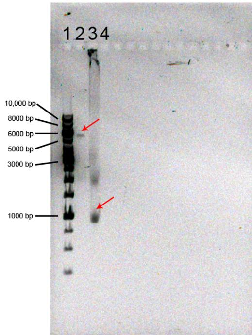
**Figure 4.16.** 1 % agarose gel for concentration determination of ligation-ready pET-11a and mut-DEFB4A-GFP, run in 1X TAE buffer at 70 V DC electrical field for 90 min. Lane 1 contains 3  $\mu$ l Generuler™ 1 kb DNA Ladder. Lane 2 contains 1  $\mu$ l ligation-ready pET-11a. Lane 3 contains 1  $\mu$ l ligation-ready mut-DEFB4A-GFP. DNA samples contain water, molecular biology reagent, to 2.5  $\mu$  and 0.5  $\mu$ l 6x DNA Loading Dye.
