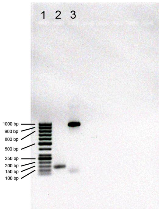
**Figure 4.11.** 1 % agarose gel for examination of mut1 and mut2 PCR products, run in 1X TAE buffer at 70 V DC electrical field for 90 min. Lane 1 contains 6  $\mu$ l Generuler™ 50 bp Plus DNA Ladder. Lane 2 contains 1  $\mu$ l mut1 PCR product. Lane 3 contains 1  $\mu$ l mut2 PCR product. DNA samples contain water, molecular biology reagent, to 5  $\mu$ l and 1  $\mu$ l 6x DNA Loading Dye.
