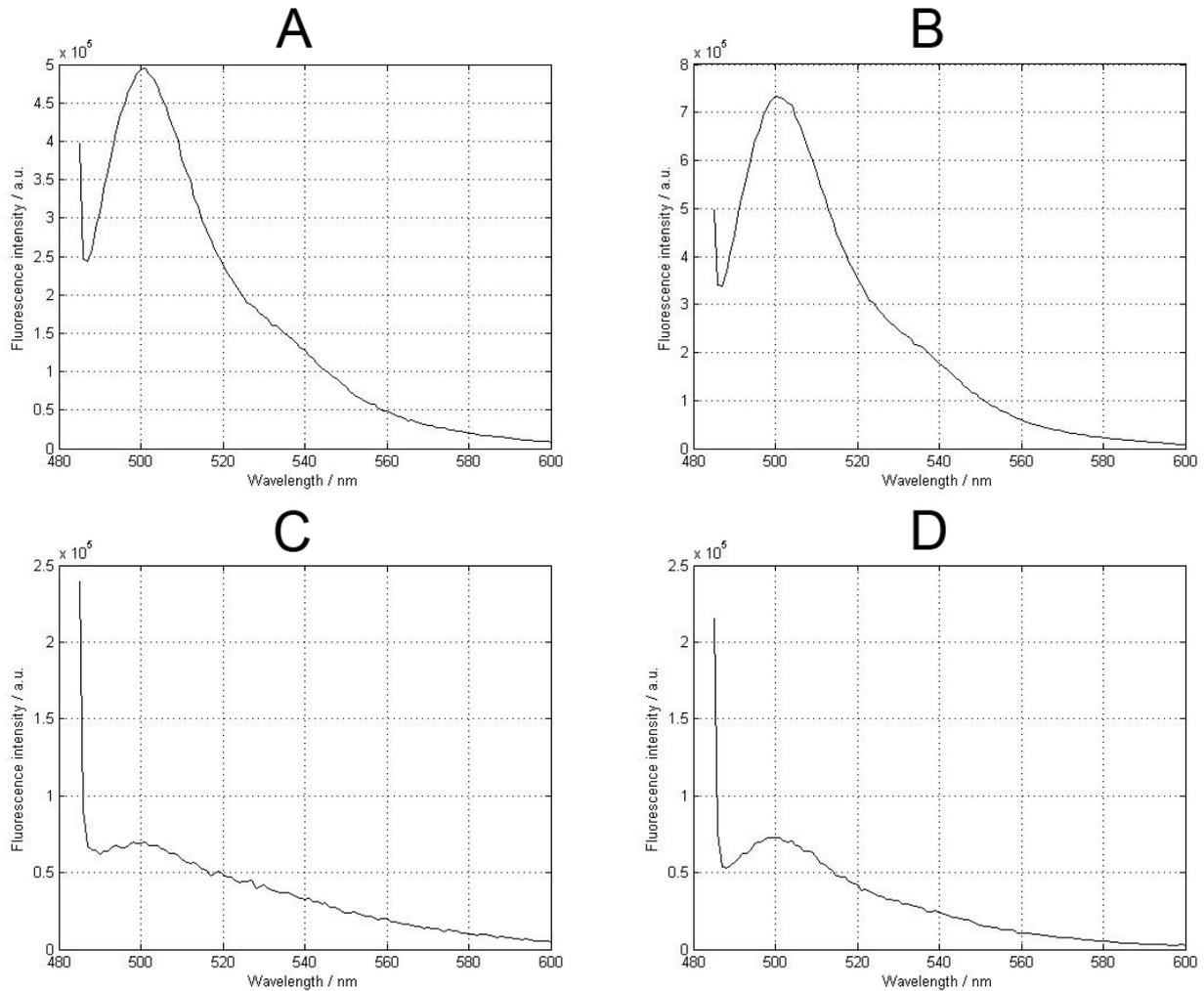
**Figure 4.22.** Fluorescence measurements of HbD-2-turboGFP fusion protein expressed in *E. coli* Origami 2(DE3) cells at 25 °C, 230 RPM. A) Induced with 0.1 M IPTG; TES fraction of protein collection protocol. B) Induced with 0.1 M IPTG; water fraction of protein collection protocol. C) Uninduced; TES fraction of protein collection protocol. D) Uninduced; water fraction of protein collection protocol.
