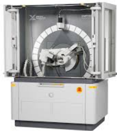
Figure 3.5: This picture depicts the Malvern Panalytical Empyrean XRD machine.[malvern Panalytical, ]
