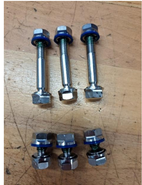
Figure 3: Top - Bolts from KB. Bottom - Bolts from Nordturn
