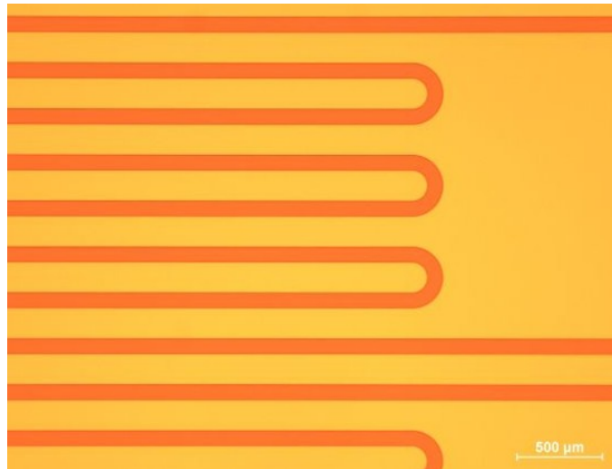
Figure 4.7: Picture of mold 1 after development, showcasing well-structured channels.
