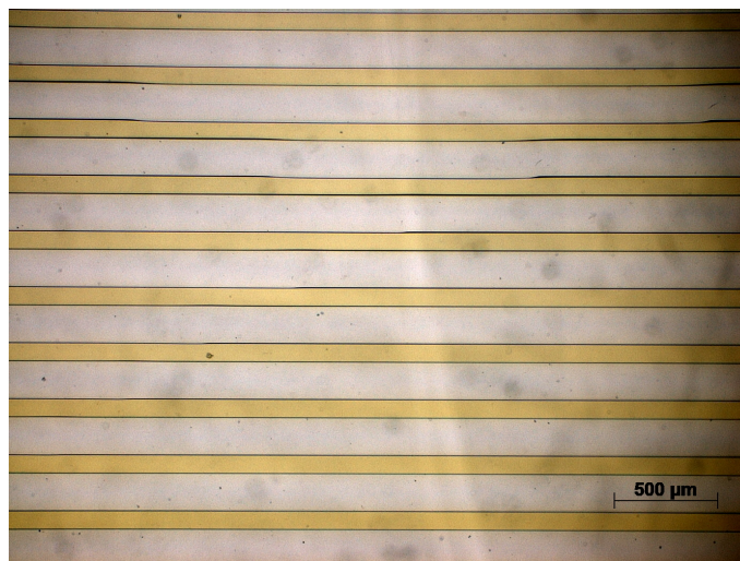
Figure 4.19: Visualization of the channel flow using fluorescein disodium salt as a dye.
