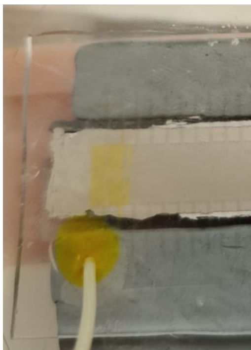
Figure 4.20: Delamination of the area around the inlet of a wafer 2 chip, when injecting with paraffin oil, at a flow rate of 5 \mu\text{L}/\text{min} .
