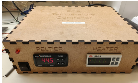
Figure 3.2: The electrical box is responsible for the electronics related to the heating.
