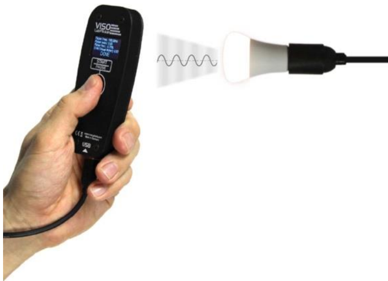
Figure 5 - LabFlicker flicker tester. Image courtesy of Viso Systems (n.d). https://www.visosystems.com/products/labflicker/ (Viso Systems - LabFlicker)
