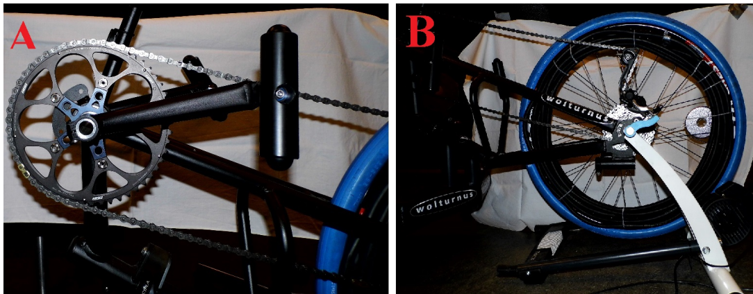
Figure 6.2: A: shows the crank-mechanism with the cranks oriented in phase of each other. B: shows the driven front wheel loaded with a 15 m 8 kg copper cable to increase the kinetic energy. A 0.5 kg weight disc is also attached to the wheel to outbalance the weight distribution.
