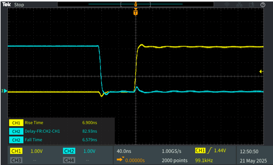
Figure 3.4: FPGA Gate control signals, showing the rise time, fall time and dead time
