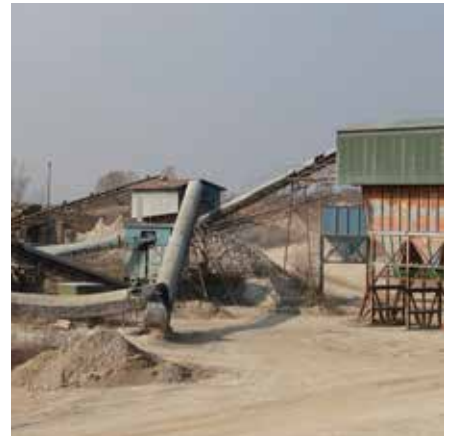
ill. 34 gravel processing plant with conveyors and hoppers
