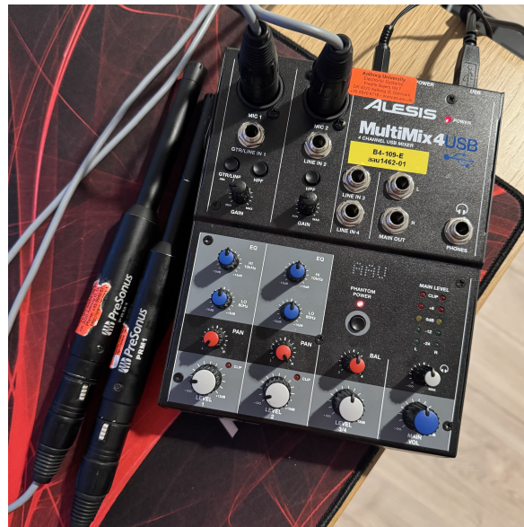
Figure A.1: Measurement setup for heart sound acquisition using PRM1 and MultiMix 4 USB
