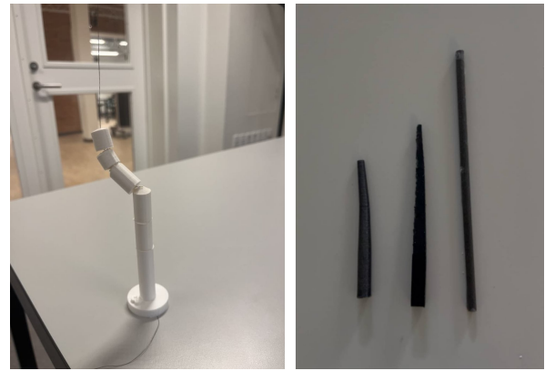
Figure 9: Picture on the left shows the modular stem, picture on the right shows the evolution of the bendable TPU stem
