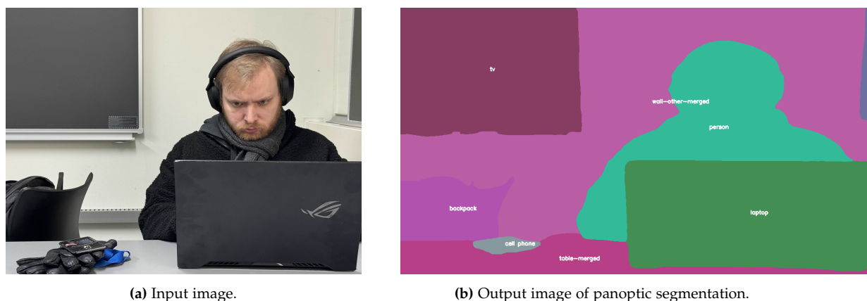
Figure 2.11: This image shows how Panoptic segmentation using both approaches to identify and labeling objects in the image.
