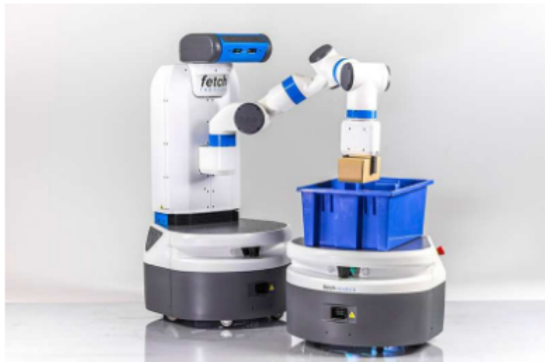
Figure 2.4: Fetch Robotics' Fetch Robot with an additional mobile base which carries items picked up by the main robot. This robot is mainly designed for working in warehouses.[8]
