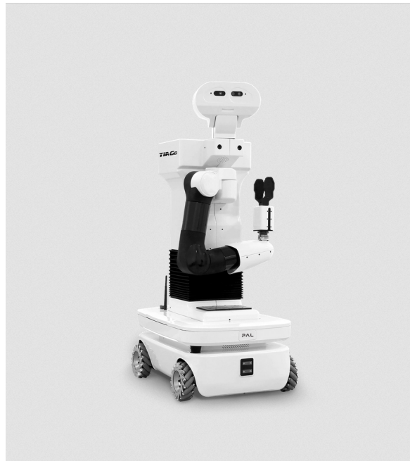
Figure 2.2: The Tiago robot with a omni directional drive base, equipped with a RGB-D camera and a 7 DOF manipulator.
