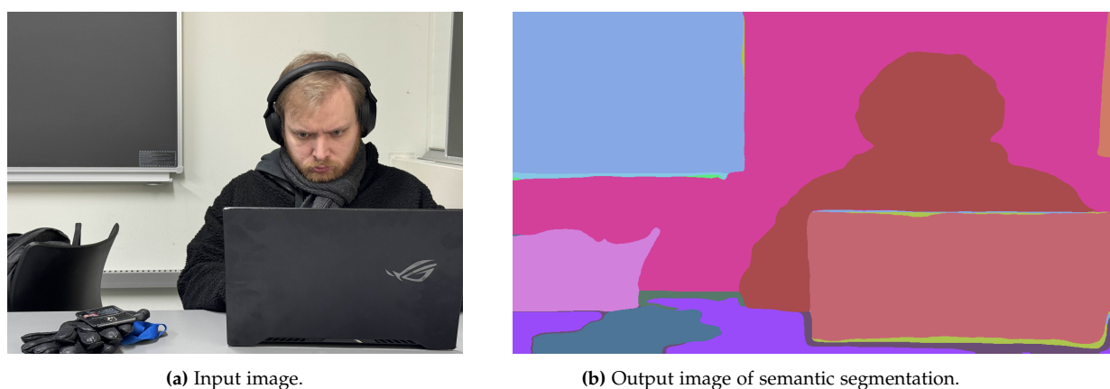
Figure 2.9: This image shows how semantic segmentation has categorised each pixel into regions based on the pixel labeling.
