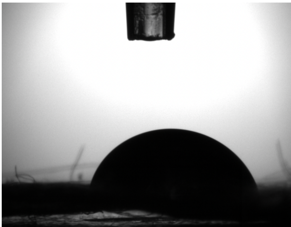
Figure 13.26. ACD 3 with a contact angle of 74.04^\circ
