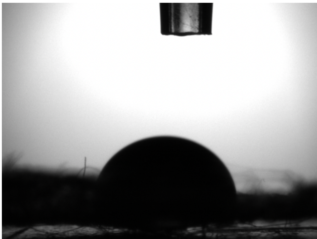
Figure 13.8. ACD 3 with a contact angle of 78.34^\circ
