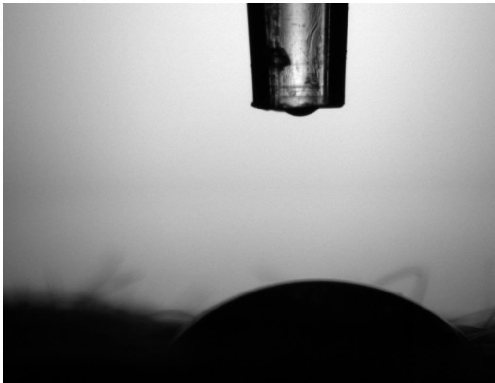
Figure 13.20. ACD 1 with a contact angle of 44.27 °
