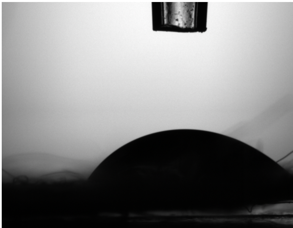
Figure 13.39. ACD 2 with a contact angle of 50.1 °
