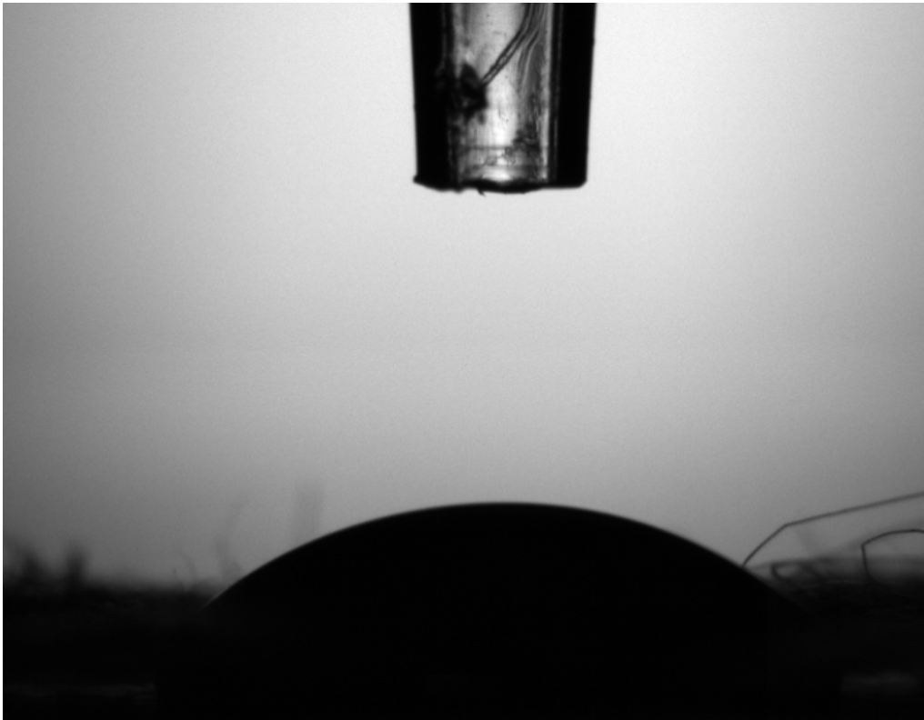
Figure 13.1. ACD 1 with a contact angle of 39.51 °
