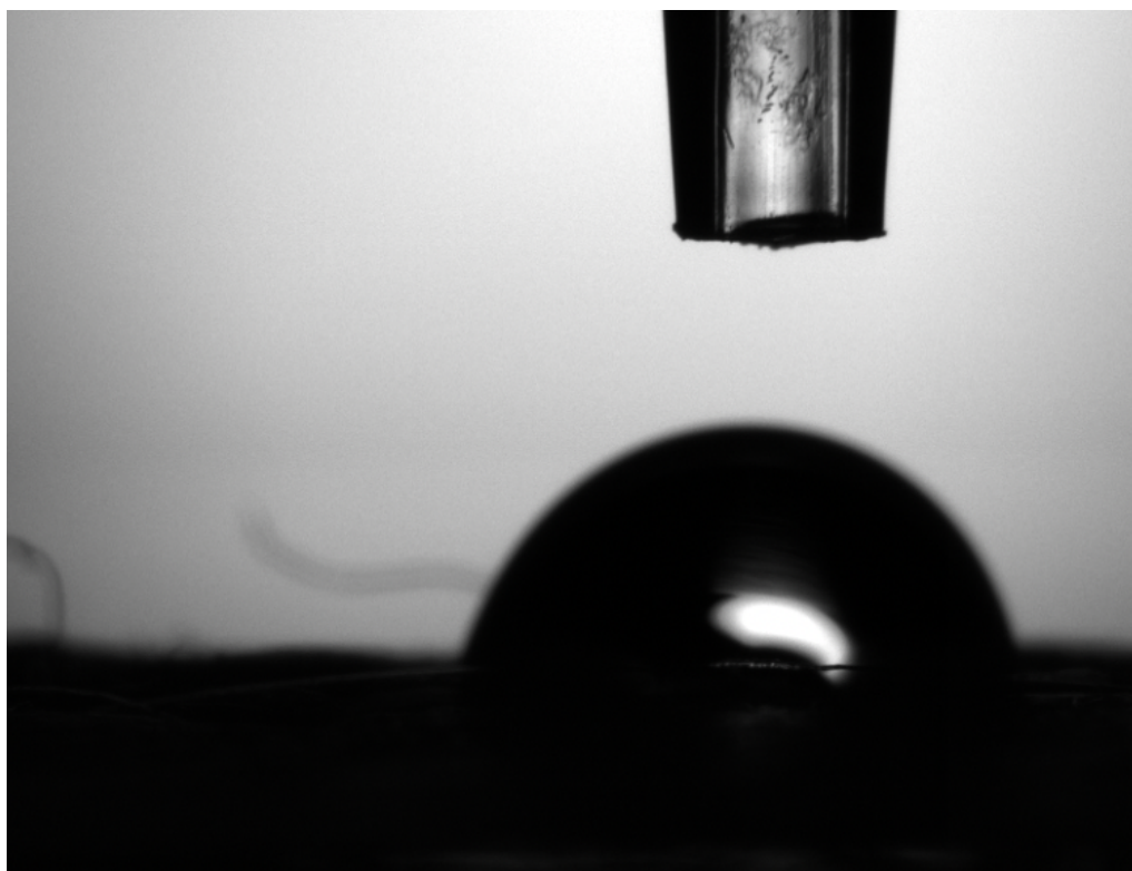
Figure 13.41. ACD 3 with a contact angle of 78.88^\circ
