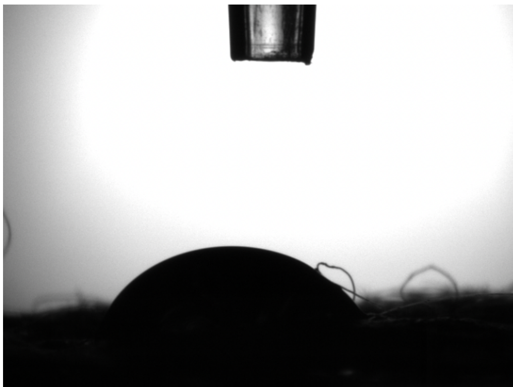
Figure 13.22. ACD 2 with a contact angle of 52.33^\circ
