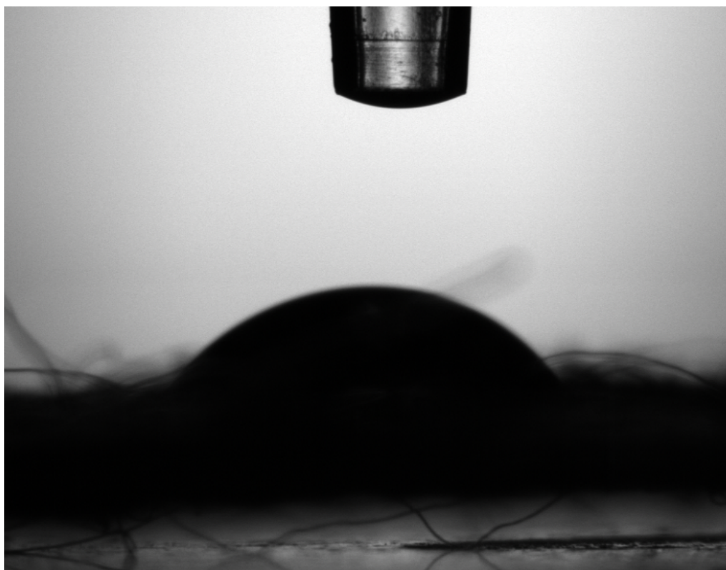
Figure 13.40. ACD 2 with a contact angle of 48.39 °
