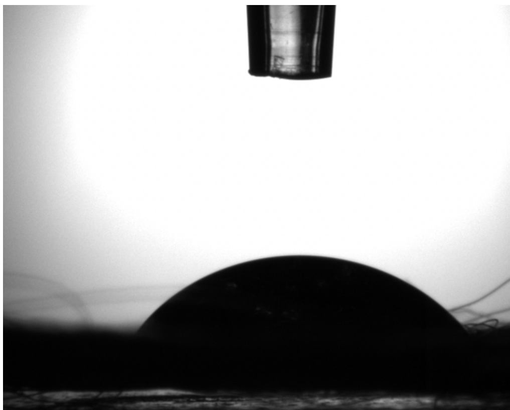
Figure 13.21. ACD 1 with a contact angle of 49.75 °
