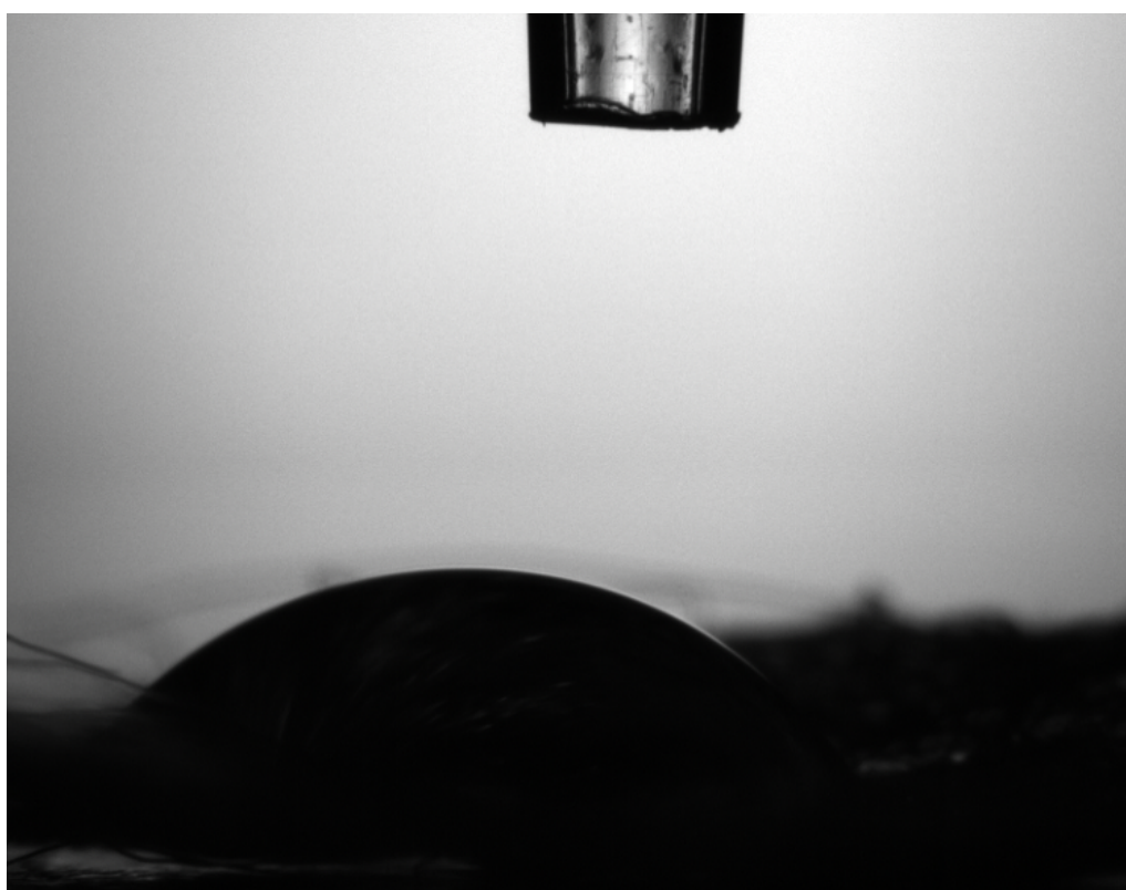
Figure 13.23. ACD 2 with a contact angle of 51.9^\circ
