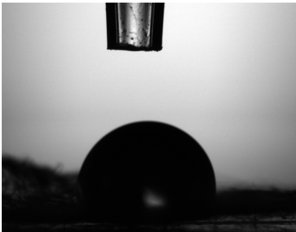
Figure 13.13. ACD 5 with a contact angle of 106.76^\circ
