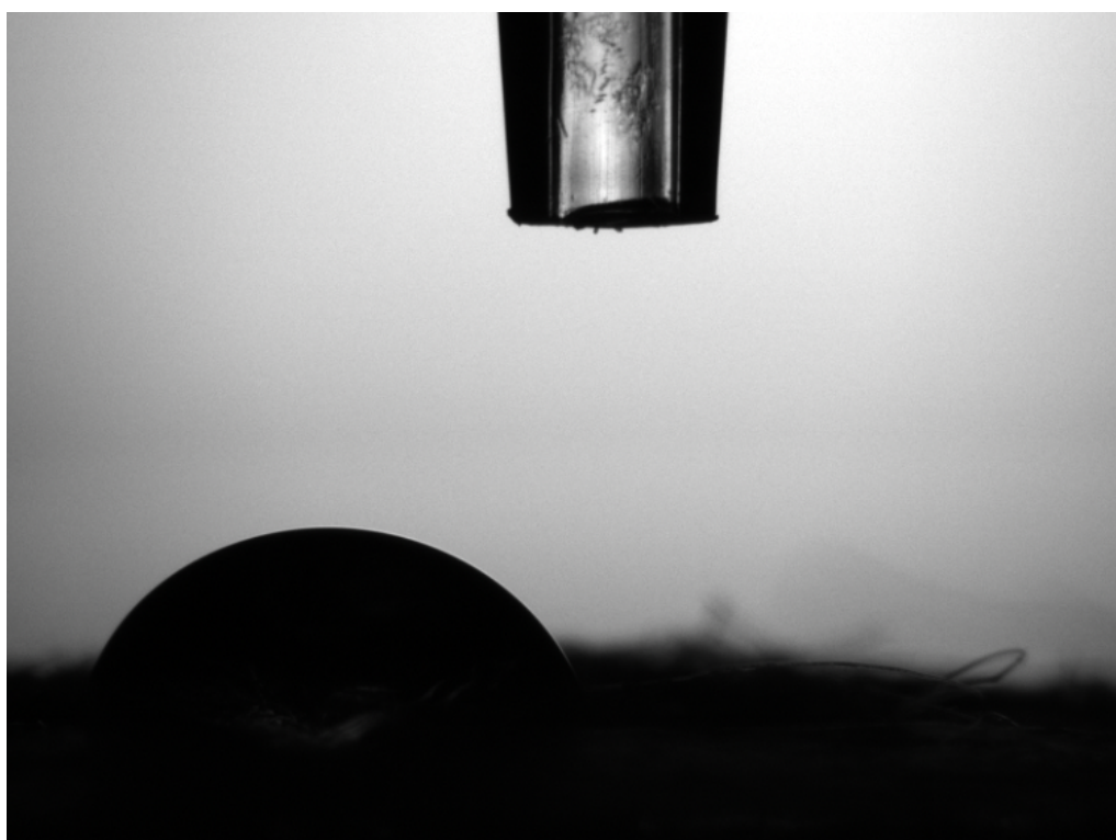
Figure 13.42. ACD 3 with a contact angle of 64.66^\circ
