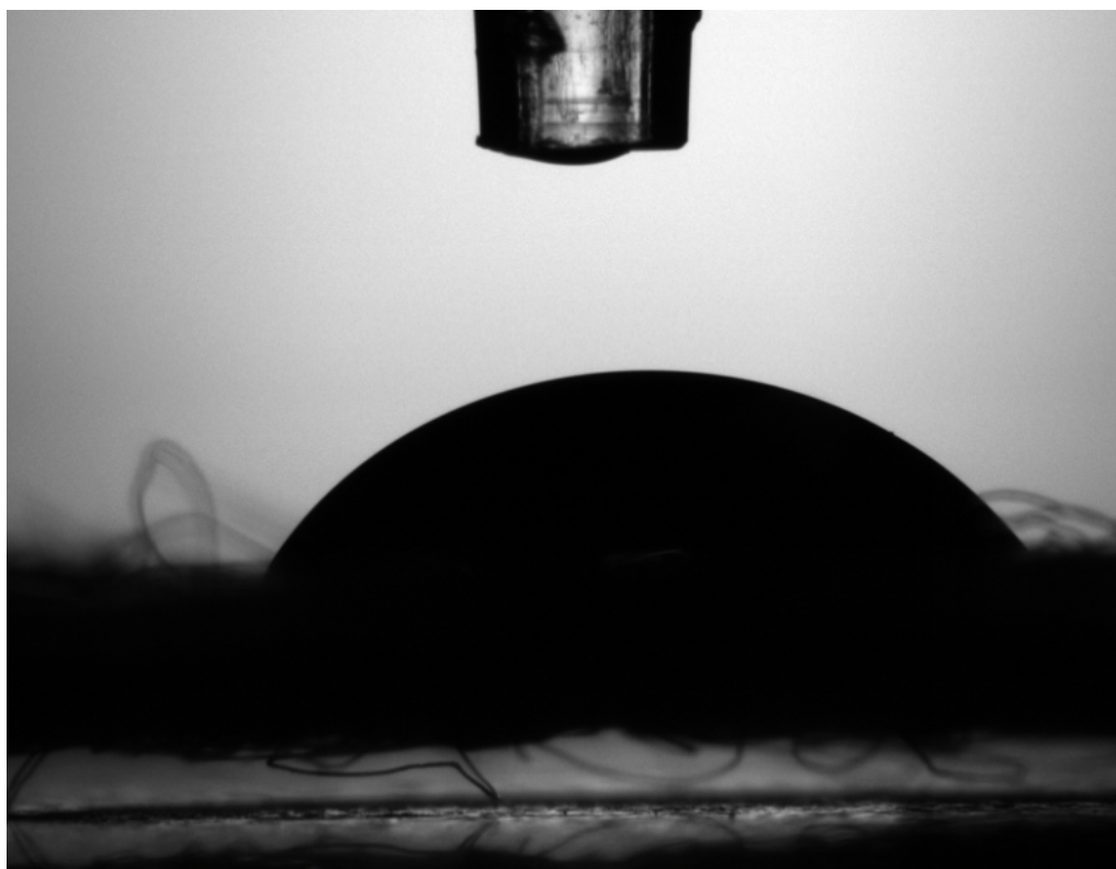
Figure 13.37. ACD 1 with a contact angle of 51.3 °
