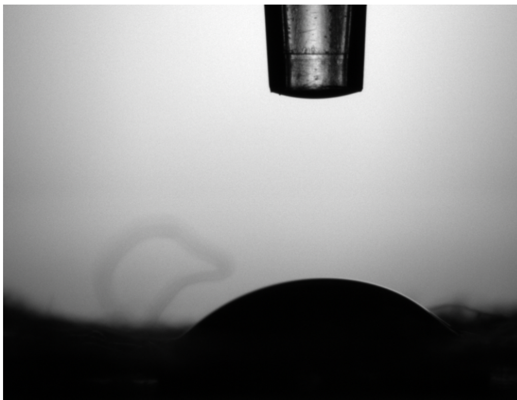
Figure 13.6. ACD 2 with a contact angle of 51.46 °
