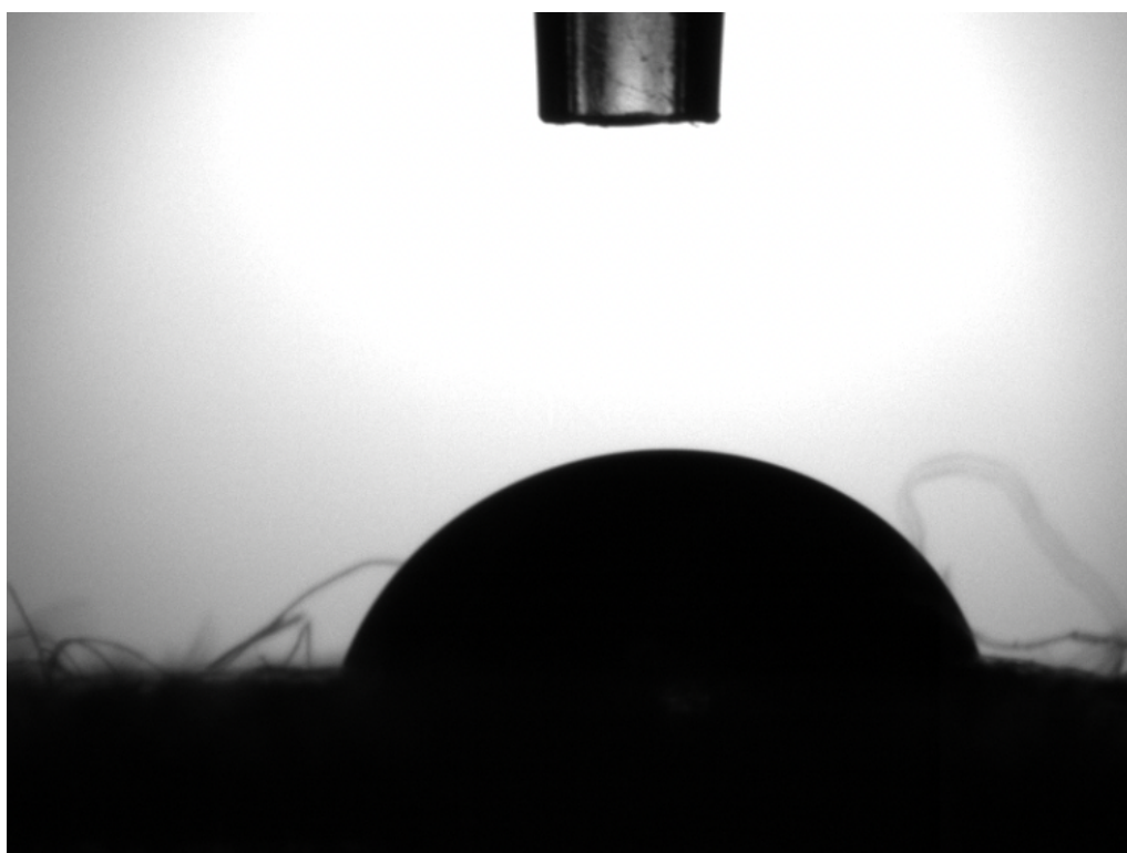
Figure 13.7. ACD 3 with a contact angle of 74.11 °
