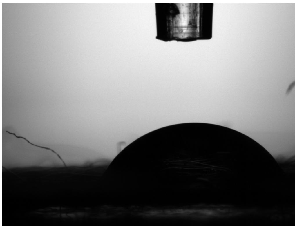
Figure 13.38. ACD 1 with a contact angle of 50.28 °
