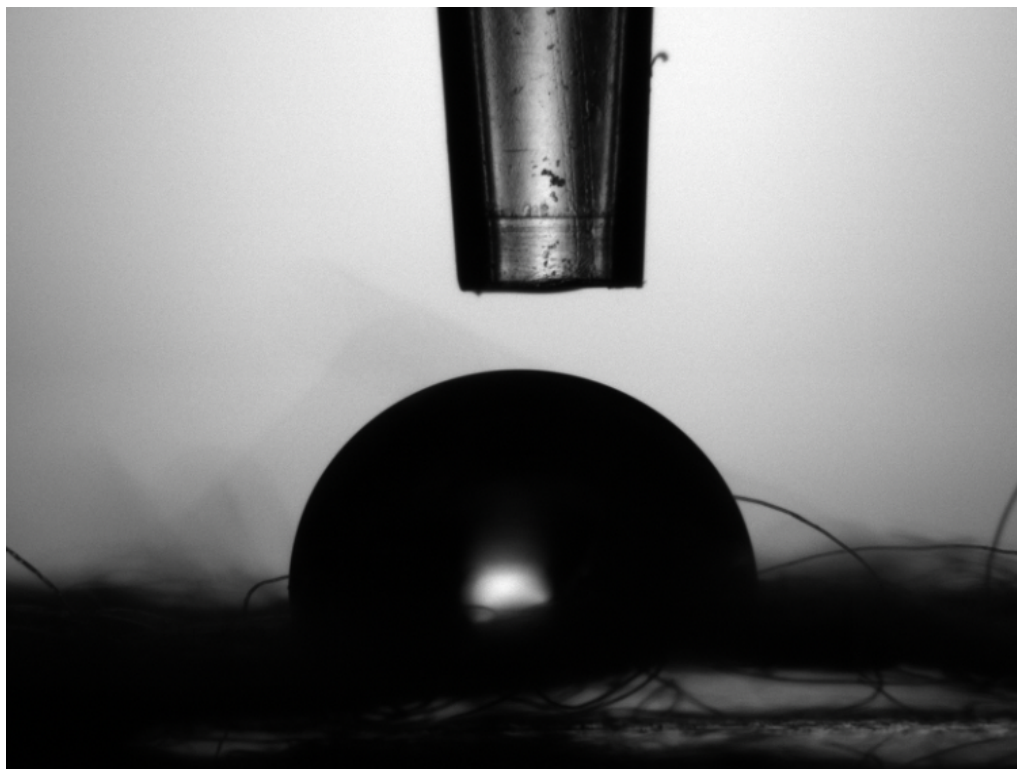
Figure 13.43. ACD 4 with a contact angle of 93.03 °
