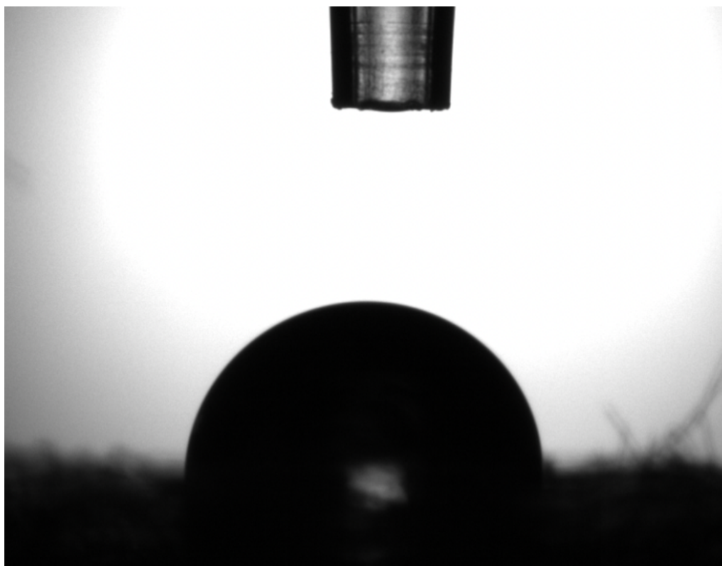
Figure 13.12. ACD 4 with a contact angle of 89.664^\circ
