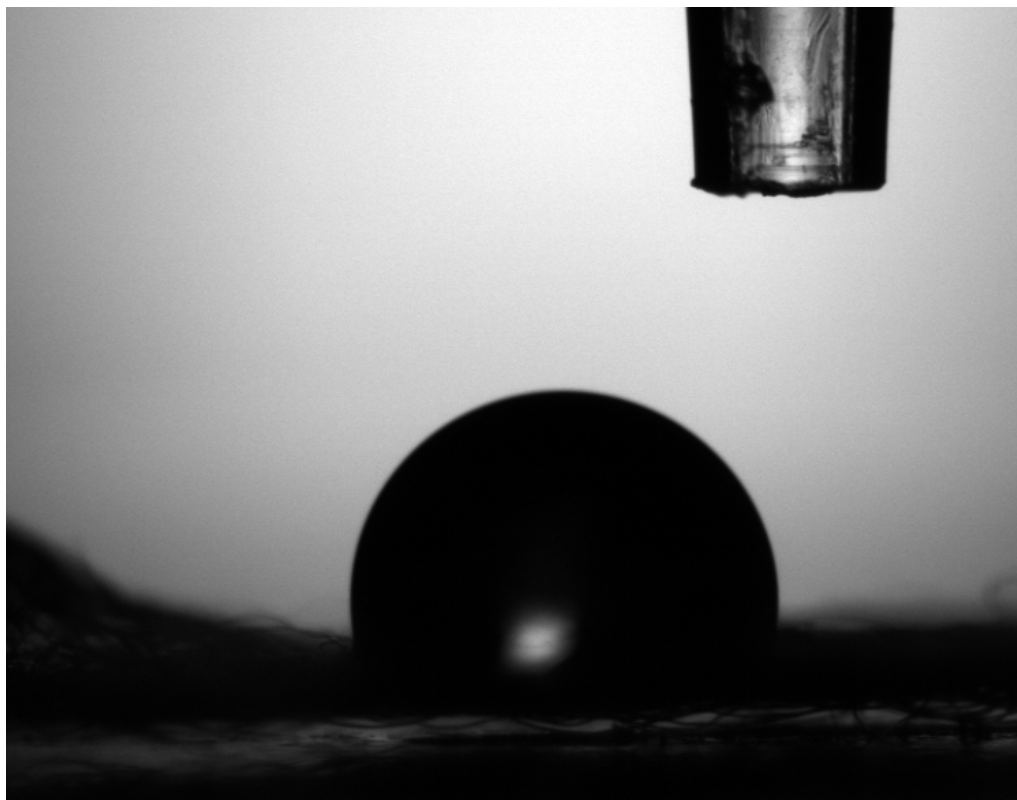
Figure 13.14. ACD 5 with a contact angle of 112.13 °
