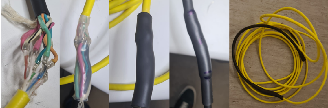
Figure 3.10: Cable Soldering & Waterproofing
