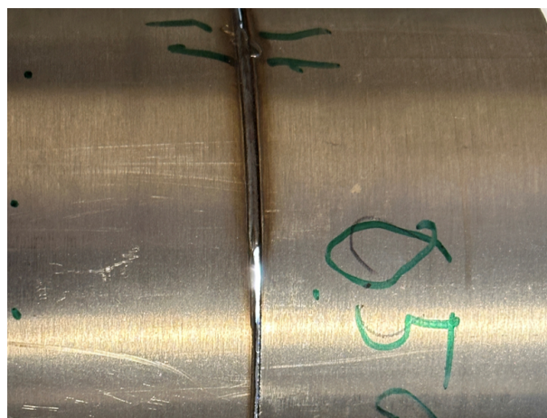
Figure 1.1 Lack of fusion in 0.5mm gap duct welding
