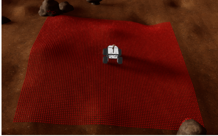
Figure 5.2: Visualization of the heightmap sensor modality in simulation. A 5 \times 5 m area with 0.05 m resolution is projected onto the terrain and transformed into the robot's frame for local perception and processing.
