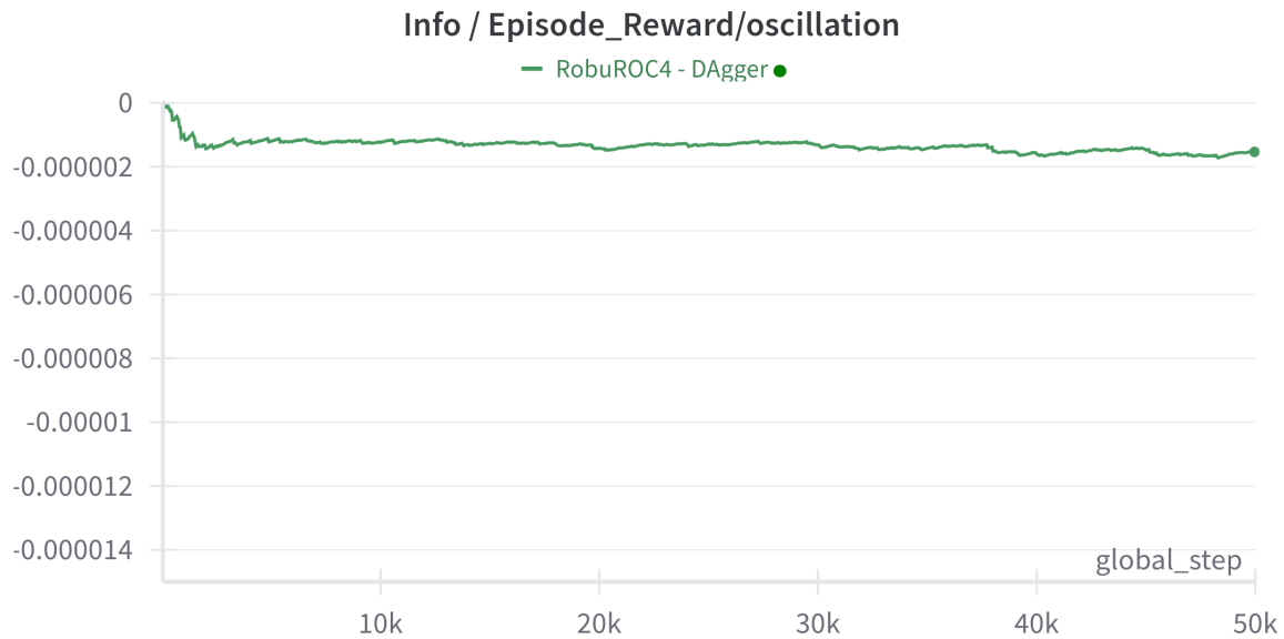
Figure 5.18: Penalty for large action changes over 50,000 evaluation steps for the RobuROC4 model trained using DAgger. The graph reflects how often and to what extent each policy exhibits erratic or unstable movements during training.
