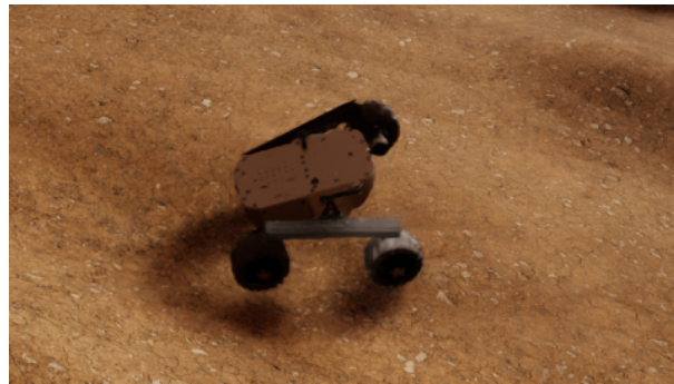
Figure 5.5: Depiction of the exaggerated movement seen during turning maneuvers for the Leo Rover, taken in Isaac Sim. As can be seen the rocker joints reach the limits in opposite directions while performing turning maneuvers.
