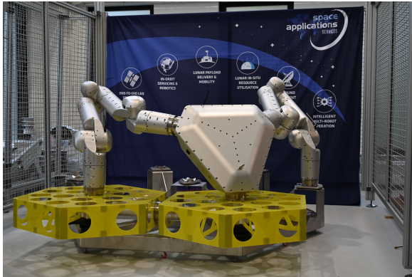
Figure 1.2: The MIRROR robot using the HOT-DOCK system to grab two structures.
