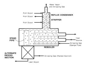
Figure 2.8: Simplified process flow diagram of stripping gas [6]
