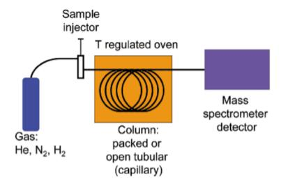
Figure 3.3: Schematic representation of a GC-MS. [26]
