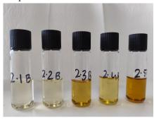
**Figure 6.8:** Thermally degraded TEG samples B with 15 wt% water contents
