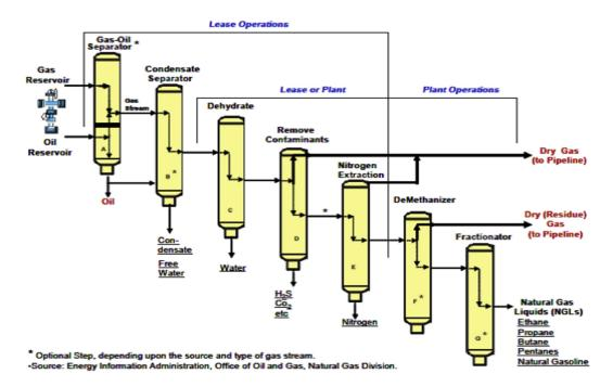
Figure 2.4: Schematic representation of general gas processing units [3].
