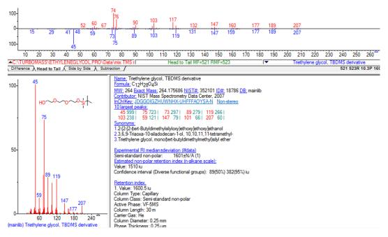
Figure 6.18: Mass spectra of TEG (1-TMS) with mass spectra of TEG (1-TMS) from a library database.
