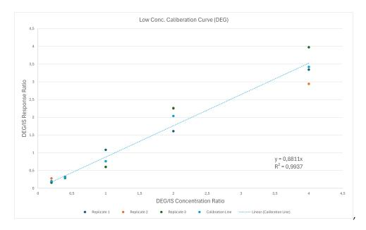
Figure 5.5: Low concentration calibration curve (DEG)
