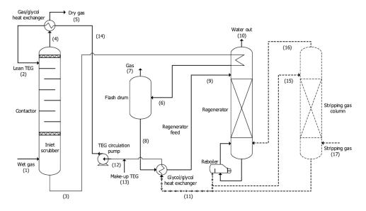
Figure 2.5: Depiction of a TEG dehydration unit with a gas stripping column. [10]
