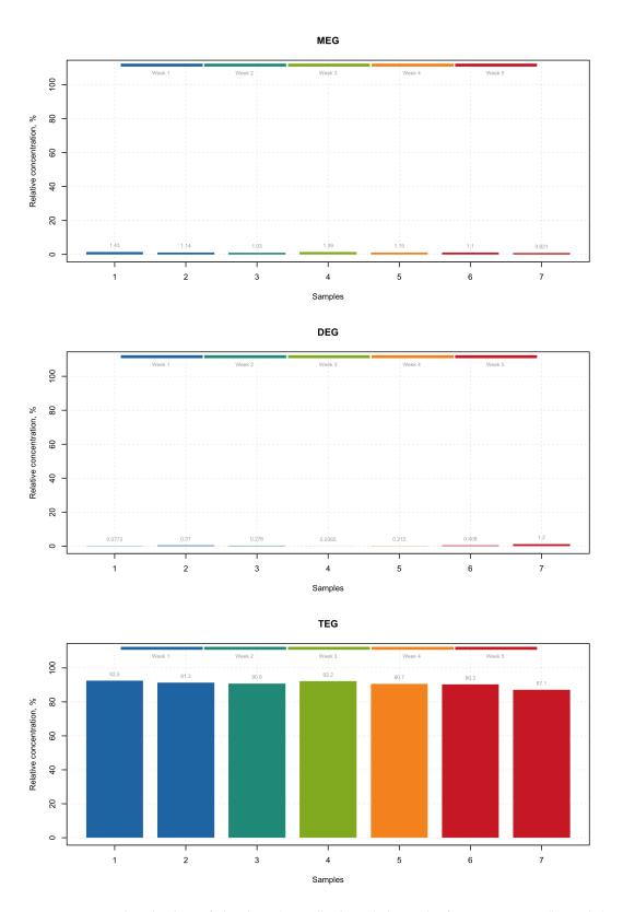
Figure 6.22: Predicted values of glycols in thermally degraded samples from experiment (by mol%).
