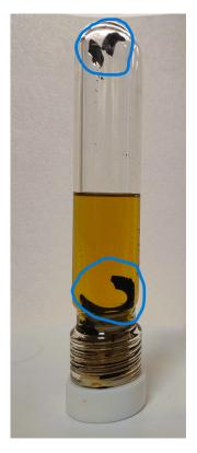
**Figure 6.9:** Detached rubber fragments of tube cap
