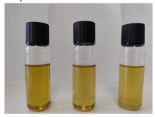
**Figure 6.4:** Thermally degraded TEG samples at 220  $^{\circ}\text{C}$
