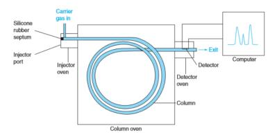
Figure 3.1: Schematic representation of a gas chromatograph. [24]
