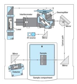
Figure 3.4: Schematic representation of a FTIR spectrometer. [24]
