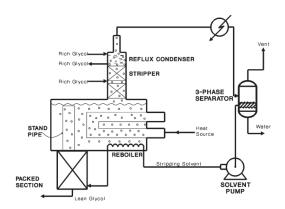
Figure 2.6: Simplified process flow diagram of DRIZO [6]
