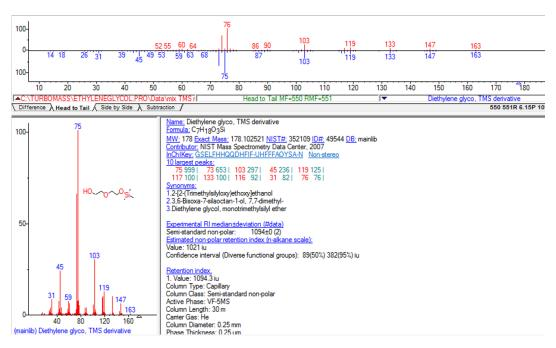
**Figure A.1:** Mass spectra of DEG (1-TMS) with mass spectra of DEG (1-TMS) from a library database.
