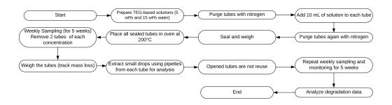
Figure 5.2: Flowchart illustrating the experimental procedure for Campaign 2.
