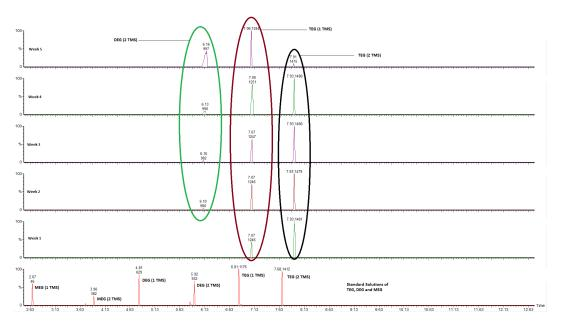
**Figure 6.16:** GC-MS chromatogram of degraded products with retention times compared to MEG, DEG, and TEG standards, showing thermal degradation of TEG at 200 °C over weeks 1–5.
