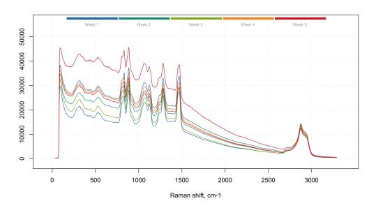
Figure 6.21: Spectra of thermally degraded samples (Raman shift plotted against intensity)
