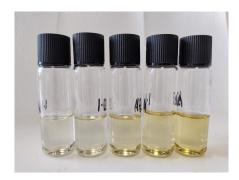
**Figure 6.5:** Thermally degraded TEG samples A with 5 wt% water contents
