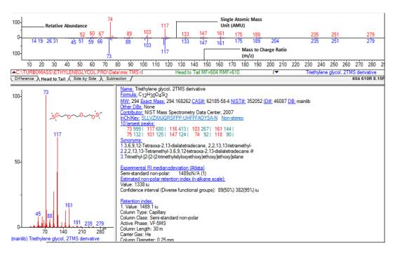
Figure 6.17: Mass spectra of TEG (2-TMS) with mass spectra of TEG (2-TMS) from a library database.
