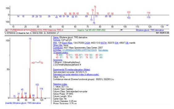
**Figure A.3:** Mass spectra of MEG (1-TMS) with mass spectra of MEG (1-TMS) from a library database.
