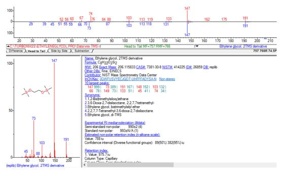
Figure A.2: Mass spectra of MEG (2-TMS) with mass spectra of MEG (2-TMS) from a library database.
