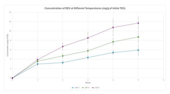
Figure 6.10: Formation of DEG in thermal degradation experiments of TEG at different temperatures.
