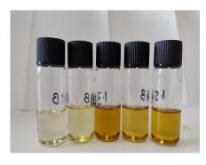
**Figure 6.6:** Thermally degraded TEG samples B with 5 wt% water contents
