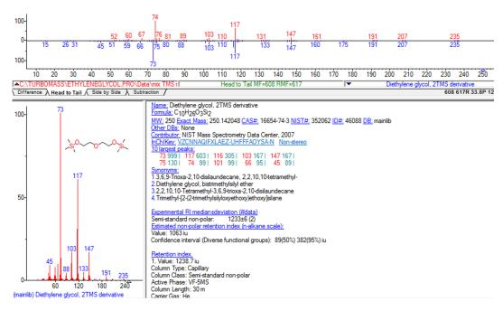
Figure 6.19: Mass spectra of DEG (2-TMS) with mass spectra of DEG (2-TMS) from a library database.
