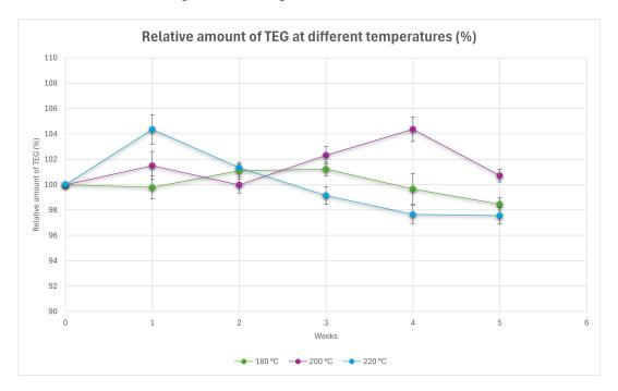
Figure 6.12: Thermal degradation of TEG at different temperatures.
