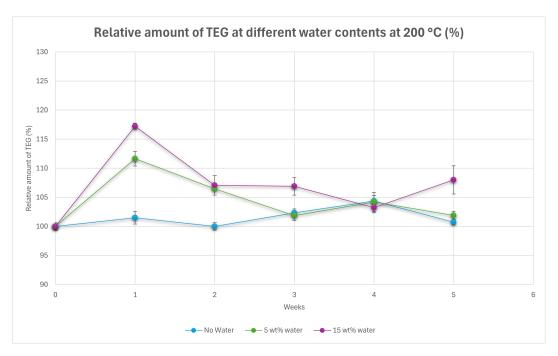
Figure 6.15: Thermal degradation of TEG at different water contents at 200 °C.
