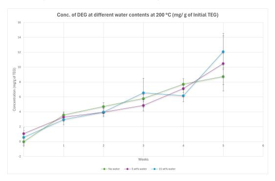
**Figure 6.13:** Formation of DEG in thermal degradation experiments of TEG at different water contents at 200 °C.
