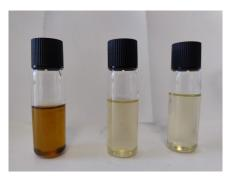
**Figure 6.2:** Thermally degraded TEG samples at 180  $^{\circ}\text{C}$
