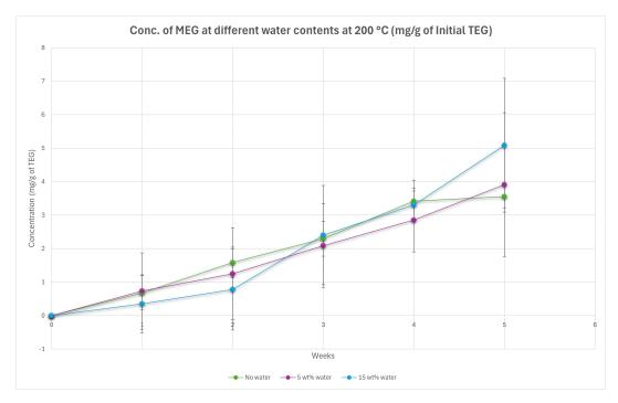
**Figure 6.14:** Formation of MEG in thermal degradation experiments of TEG at different water contents at  $200 \,^{\circ}$ C.
