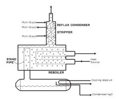
Figure 2.7: Simplified process flow diagram of COLDFINGER [6]
