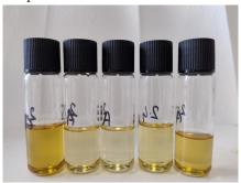
**Figure 6.7:** Thermally degraded TEG samples A with 15 wt% water contents
