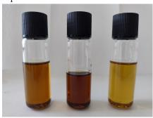
**Figure 6.3:** Thermally degraded TEG samples at 200  $^{\circ}\text{C}$
