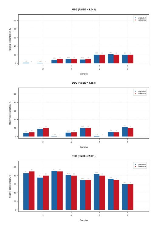
Figure 5.8: Predicted and reference values of glycols obtained from synthetic mixtures.
