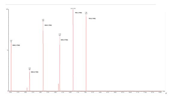
**Figure 5.7:** GC-MS chromatogram showing references of TMS-derivatized monoethylene glycol (MEG), diethylene glycol (DEG) and triethylene glycol (TEG) with their retention times.
