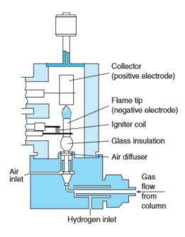
Figure 3.2: Flame ionization detector. [24]
