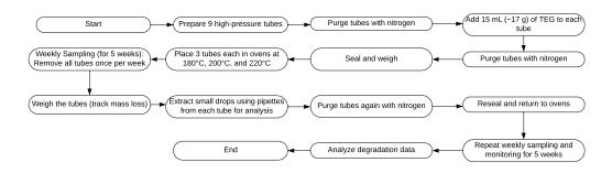
Figure 5.1: Flowchart illustrating the experimental procedure for Campaign 1.
