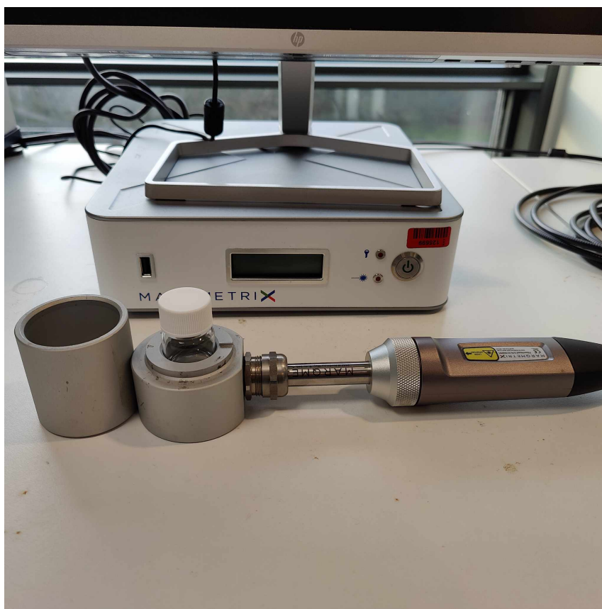
Figure 6.5: The Raman probe in the cell
