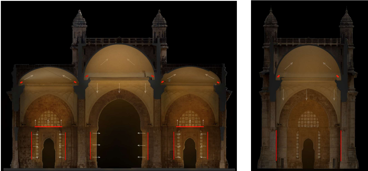
Fig 9.8 A & B : Sectional illustration of light placement and distribution across domes, arches, and jali screens, author 2025 Source : CyArk - section drawings
