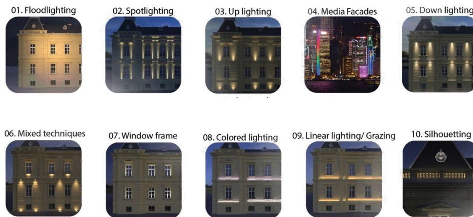
Fig 3.3 : Typologies of façade lighting techniques (Tomasovits et al.,2025)
