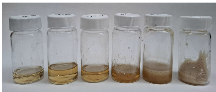
Figure 4.7: Different % w/v RP-P1 solution in 30% wt acetic acid solution. From left to right a) 15% w/v, b) 30% w/v, c) 50% w/v, d) 70% w/v, e) 90% w/v and h) 100% w/v.
