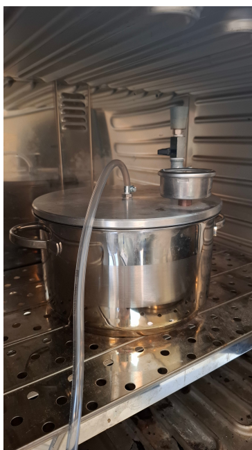
Figure 4.10: The pressure container for up-concentrating the solution under vacuum.
