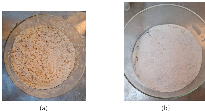
Figure 3.3: (a) recycled polymer washed once in 10 wt% NaOH solution and then rinsed with DI water; (b) recycled polymer washed once in 10 wt% NaOH solution, then rinsed 8 times with DI water, then air dried.
