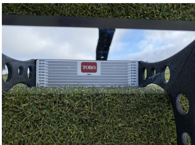
(b) The mirror on the grass prism where the grass and scale are seen.
