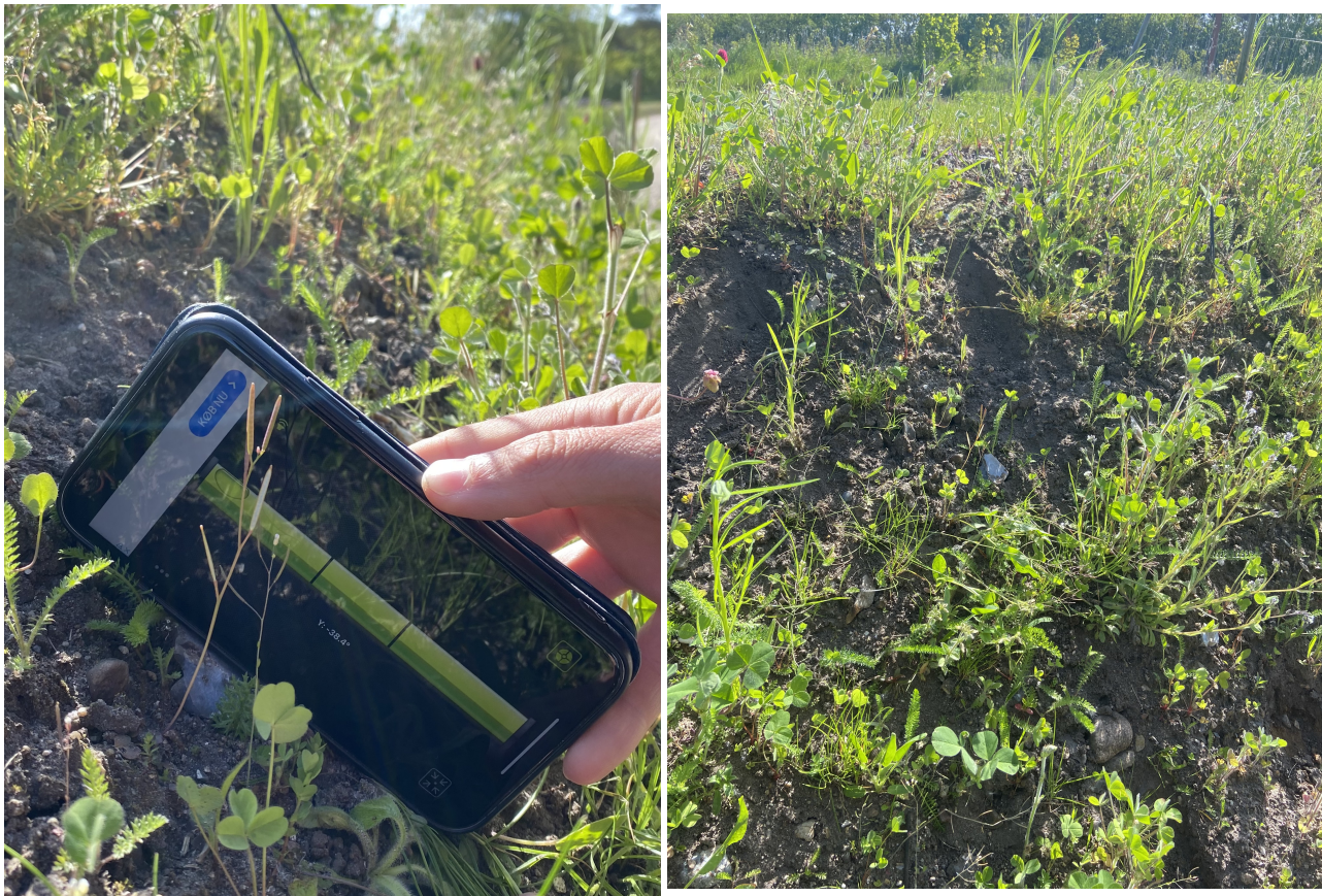
(b) Wheel marks from the mower climbing the approximately 80 % grade successfully.
