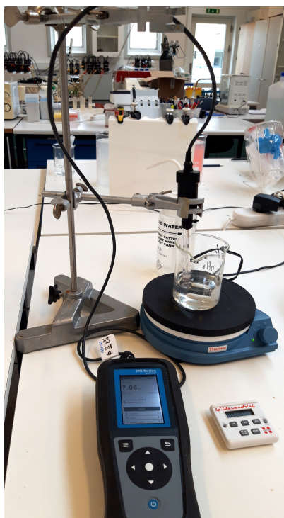
Figure 3.2: Fenton Oxidation setup: 40% COD reduction with acidic pH
