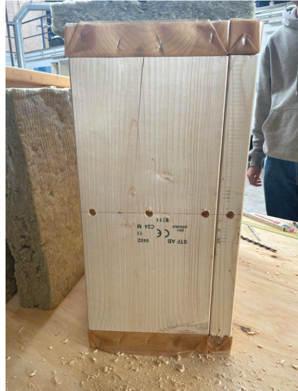
Figure C.22. Side view of the element, with holes drilled for the sensor cables.
