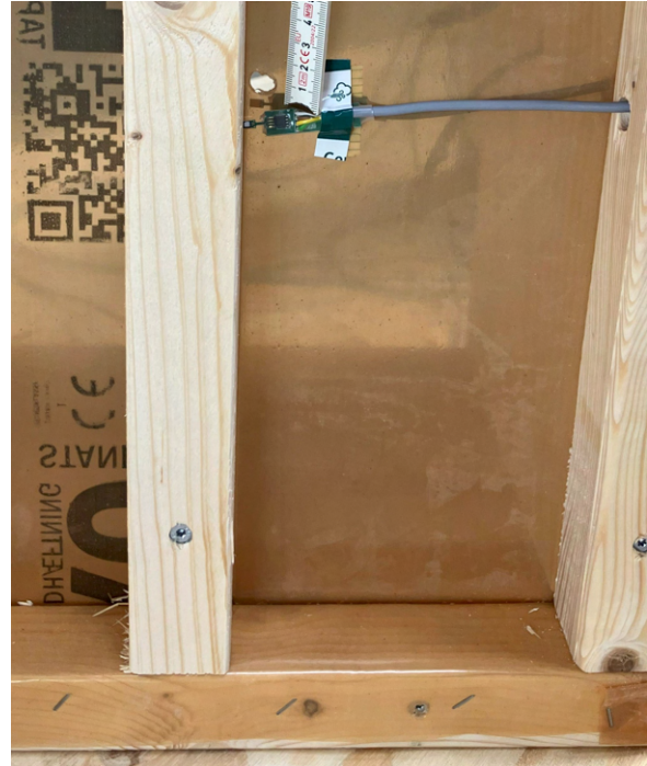
Figure C.26. PE-foil perforation in element RW-TPE at the timber stud.
