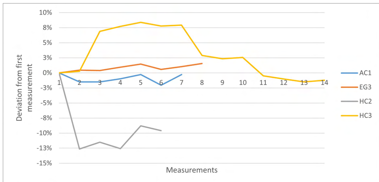
Figure T.12. Deviation in air permeability for a series of consecutive measurements.
