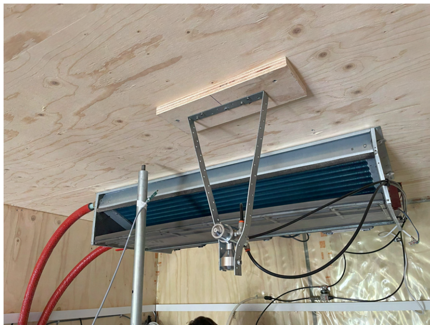
Figure 4.7. Humidification system with water mist nozzle, placed in front of the airstream from the fan coil.
