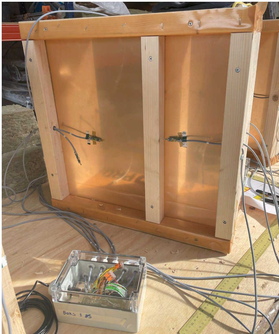
Figure C.11. Element with PE-foil and sensors placement in the installation layer.
