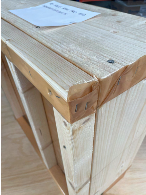
Figure C.21. Close-up of the clamped joint between the installation layer, the wall's vapour barrier and the core insulation layer.
