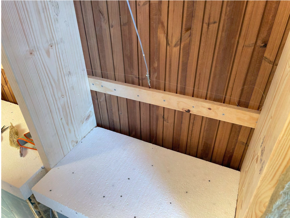
Figure C.18. Mounting of sensor in ventilated cavity
