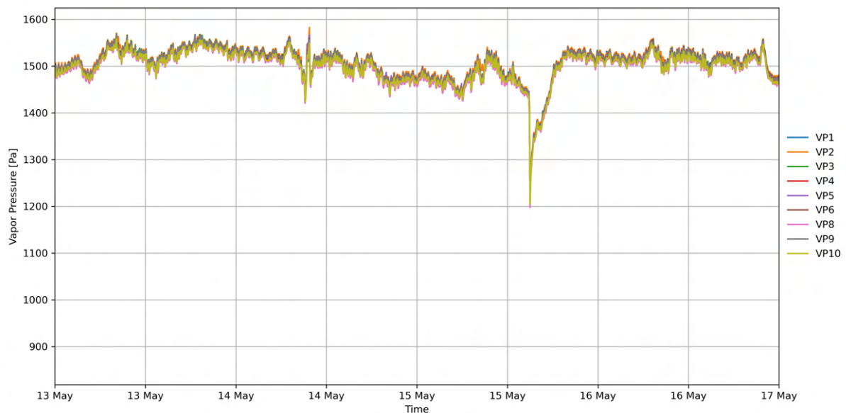
Figure A.24. The vapour pressure inside of the climatic chamber.
