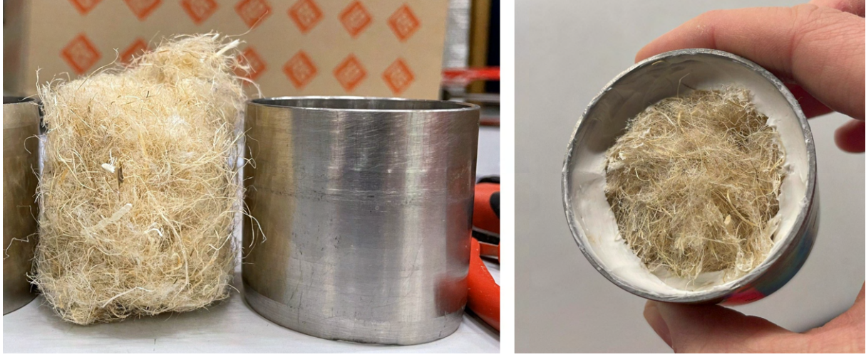
Figure T.7. Hempfiber sample ring prepared for measurements of air permeability and oxygen diffusion.
