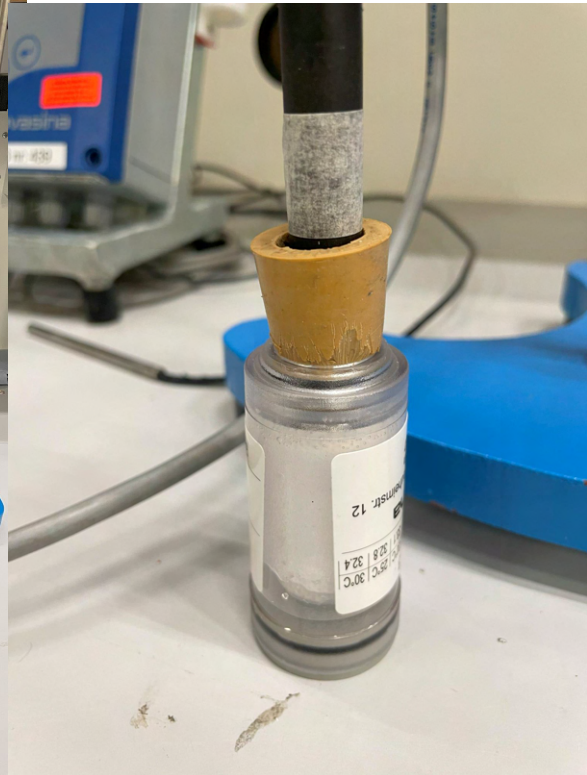
Figure V.2. Close up of the probe attached to a calibration salt.
