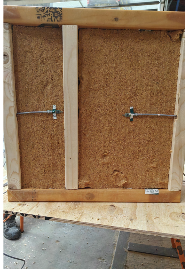
Figure C.17. Photo showing the sensors placed just behind the wind barrier.
