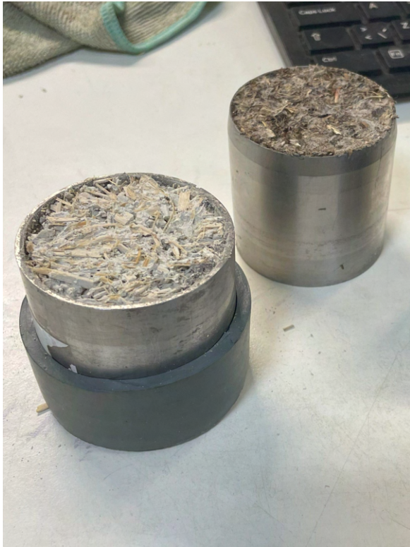
Figure T.4. Our sample ring with a rubber conical casket mounted.
