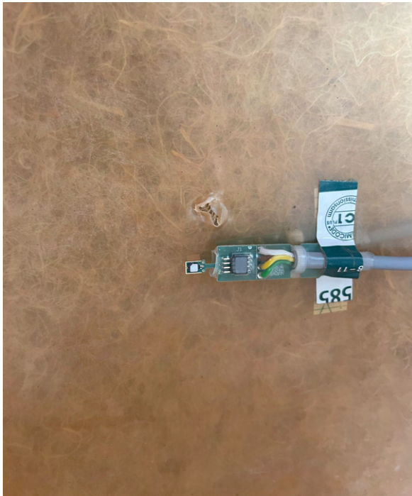
Figure C.27. PE-foil perforation in element HFI-TPE in the middle of the wide insulation layer.
