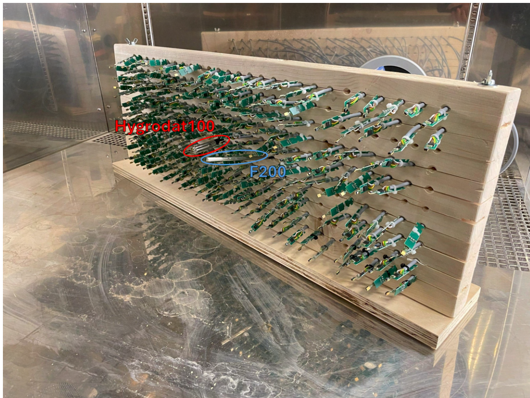
Figure E.2. Sensor mount inside climatic chamber
