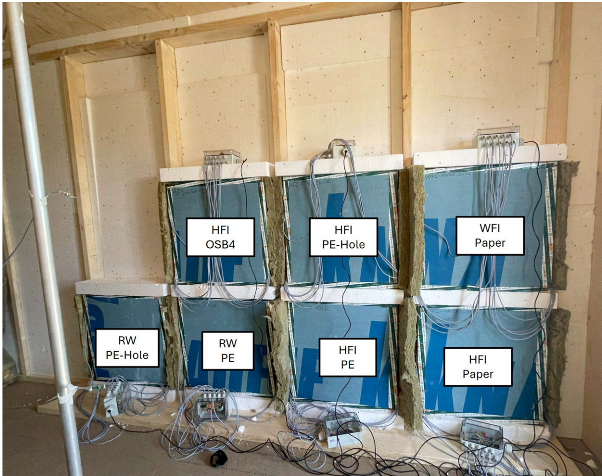
Figure A.13. Photograph of the measurement setup, with our seven wall elements in place.
