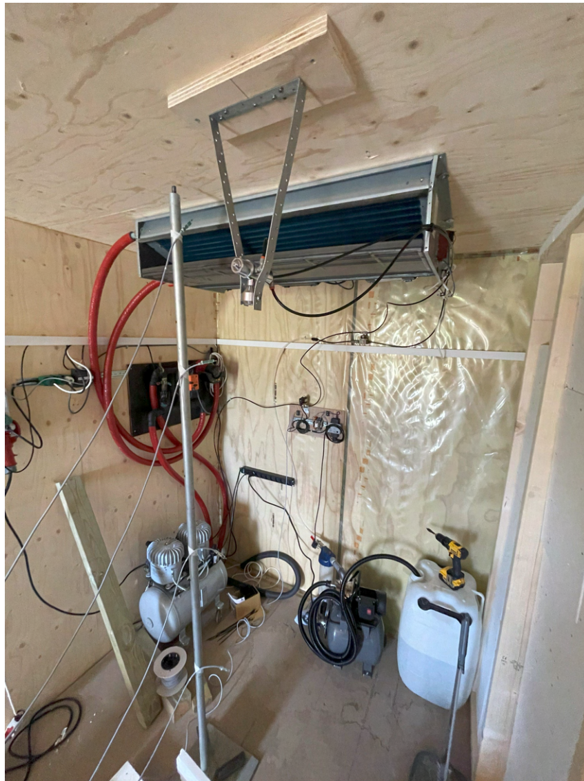
Figure A.19. Humidification system with water mist nozzle, self-contained water pressure system and water tank.
