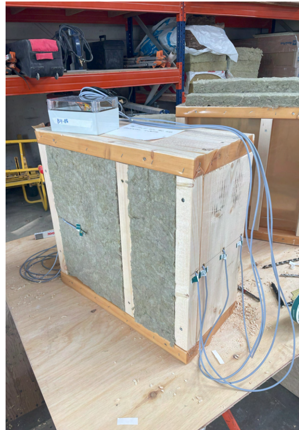
Figure C.13. Photo showing the sensor placed in the insulation measurement column, just behind the interior cladding. Photo showing the sensor placed in the installation layer. in front of the OSB4 water vapour barrier.
