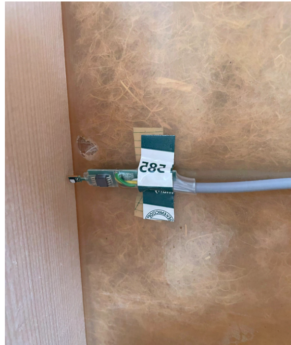
Figure C.28. PE-foil perforation in element HFI-TPE at the timber stud.
