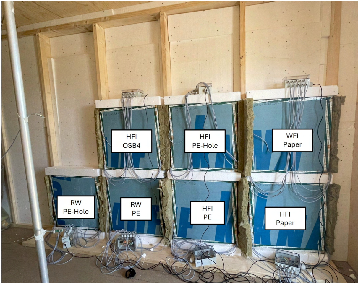
Figure 4.16. Interior view of measurement setup with wall elements.
