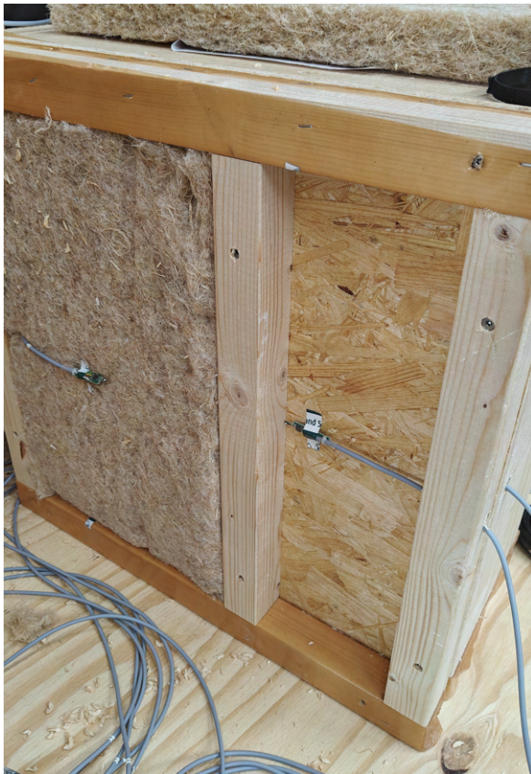
Figure C.12. Photo showing the sensor placed in the installation layer. in front of the OSB4 water vapour barrier.
