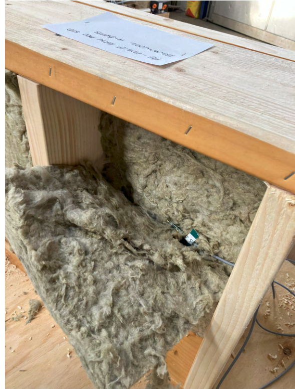
Figure C.15. Photo showing the sensor placed in the insulation measurement column, just behind the interior cladding.
