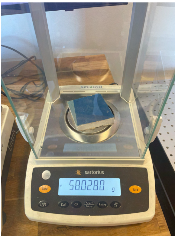
Figure R.2. Weighing of the gypsumboard
