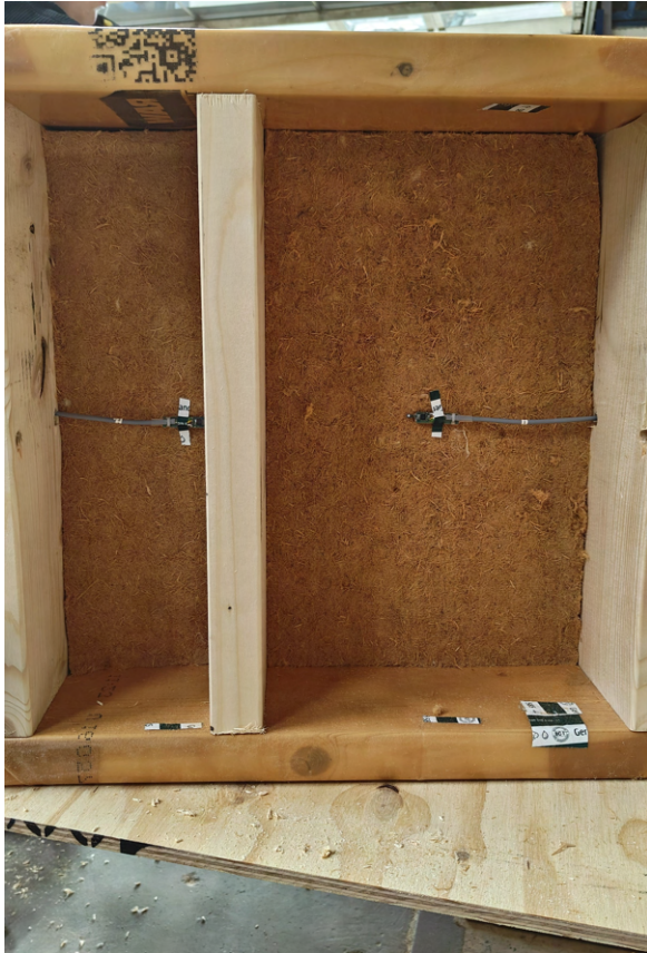
Figure C.16. Photo showing the sensors placed in the middle of the core insulation layer.
