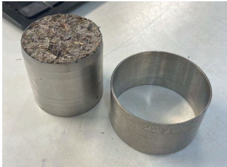
Figure T.3. Sample rings. Our sample ring to the left, and to the right the sample ring used at Aarhus University Foulum.
