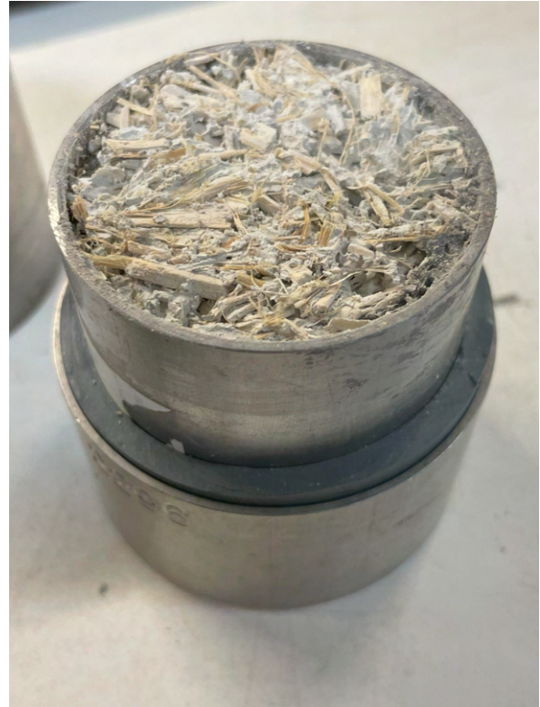
Figure T.5. Our sample ring with rubber conical casket, inside the sample ring used at AU Foulum.
