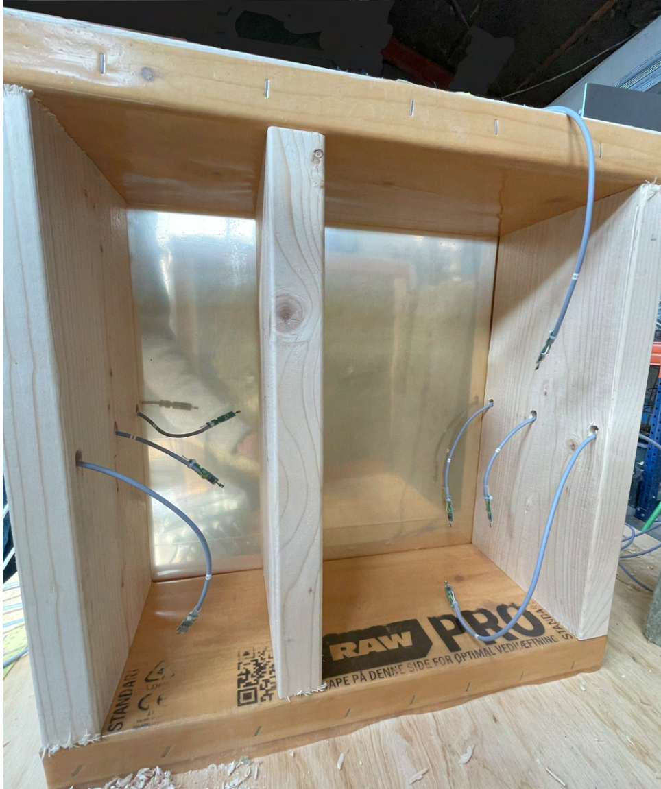
Figure C.20. Element with PE-foil, showcasing how the top and bottom is wrapped with foil. Here the sensor cables are pulled through the holes into the element.
