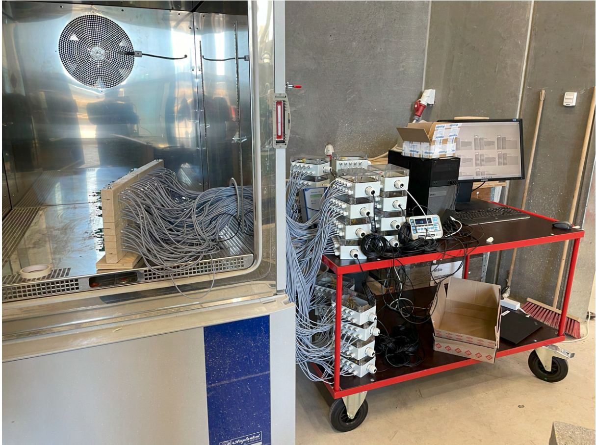
Figure E.1. Calibration setup with sensors and climatic chamber.
