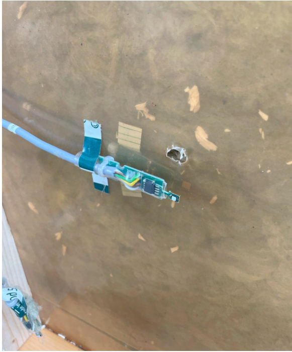
Figure C.25. PE-foil perforation in element RW-TPE in the middle of the wide insulation layer.
