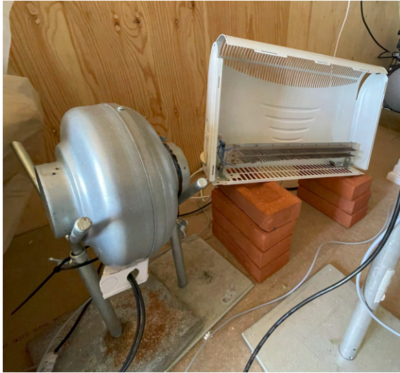
Figure 4.5. Electric heater and mixing fan inside climatic chamber.
