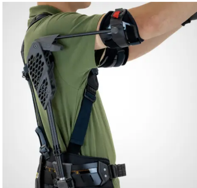
Figure 2.5: HAPO UP exoskeleton. Taken from[8]
