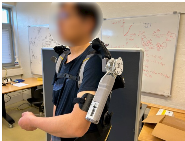
Figure 2.10: Passive shoulder exoskeleton equipped with VSM. Taken from [16]
