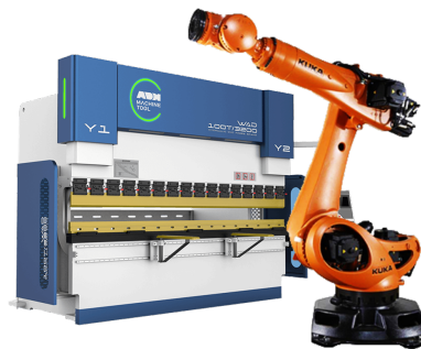
Figure 7.5: Press brake and robot needed for an automated conventional forming only setup.
