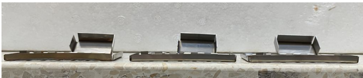
Figure B.3: Results from varying dwell times and external cooling. From left to right: (1) 3-second cooling time with excessive warping and significant thermal distortion, (2) 6-second dwell time with increased external cooling resulting in notable reduction of warping and minimal distortion, and (3) 8-second dwell time with similar cooling, showing no significant improvement compared to the second test.
