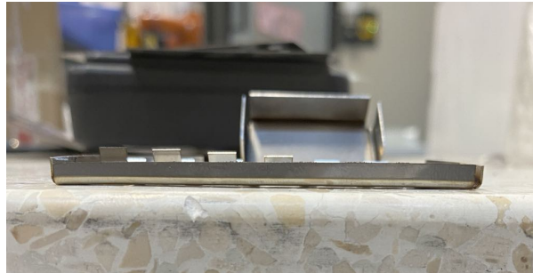
Figure 6.10: Test conducted with new bend pass sequence, less warping can be seen against the flat table.
