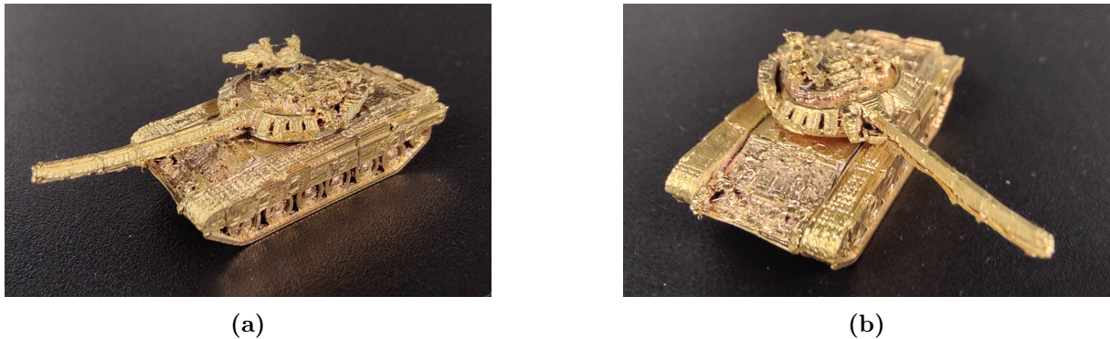
Figure 6.1. Images of gold plated 3D printed T72 tank with rotatable turret rotated (a) 0 degrees, and (b) 45 degrees
