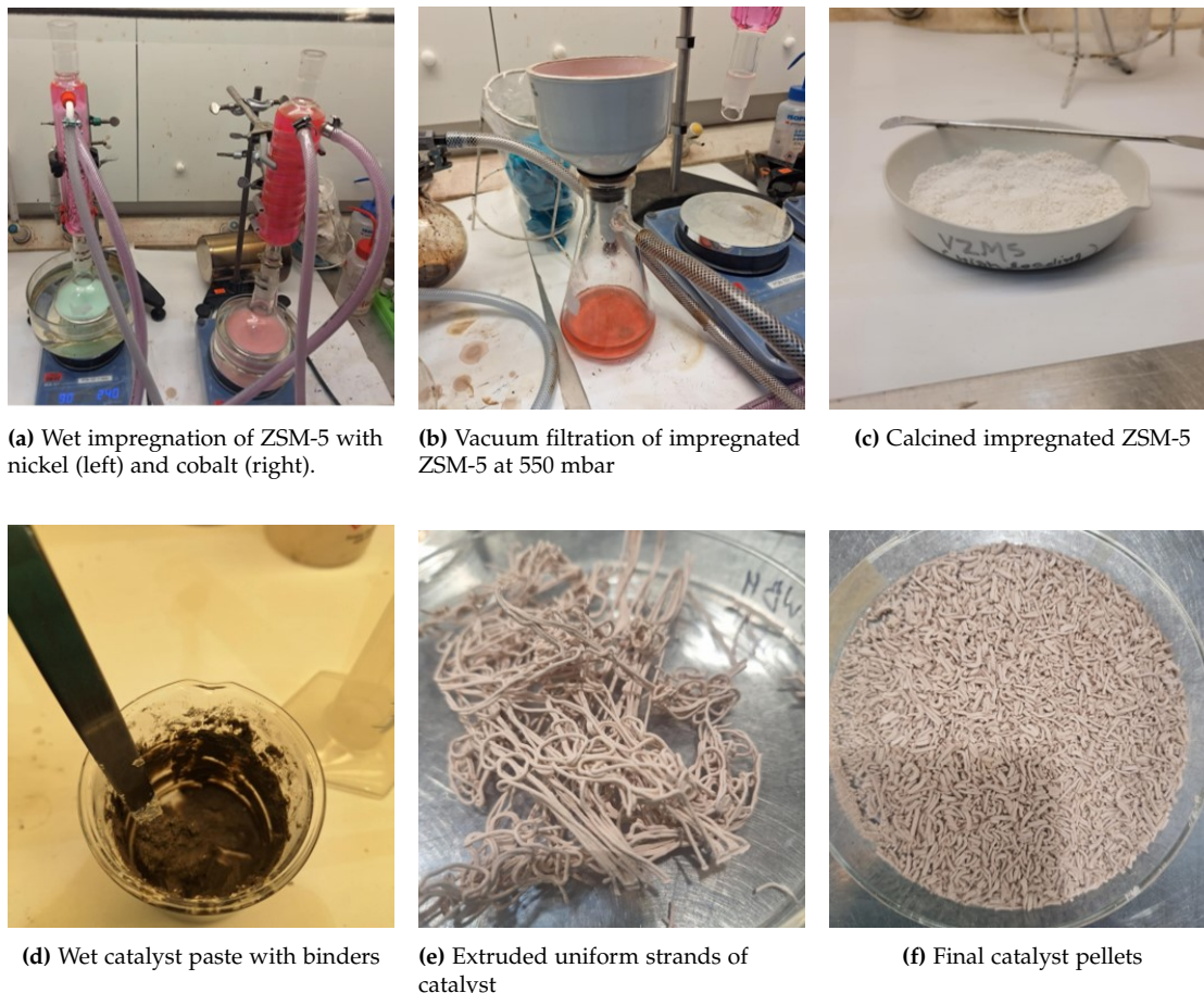
Figure 5.2: Complete catalyst synthesis procedure.
