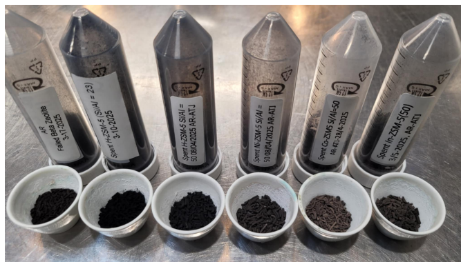
Figure 6.9: Spent catalyst of the experimental campaigns of Beta-zeolite, H-ZSM-5(23), H-ZSM-5(50), Ni-ZSM-5(50), Co-ZSM-5(50) and In-ZSM-5(50)
