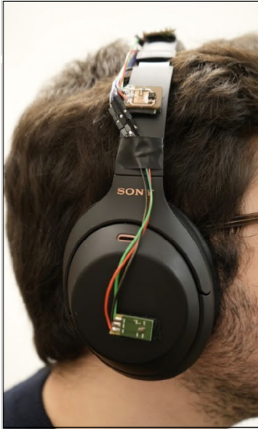
(a) Picture of the microphones mounted on a pair of headphones.
