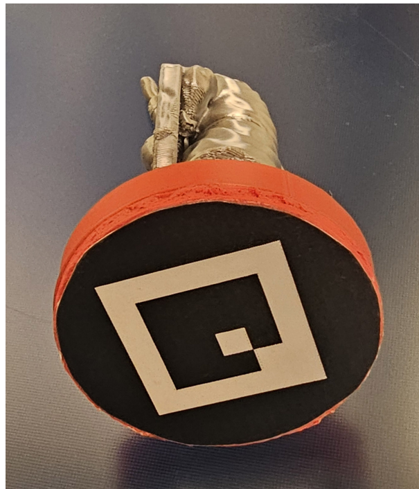
Figure 6.6: Picture of a fiducial marker.
