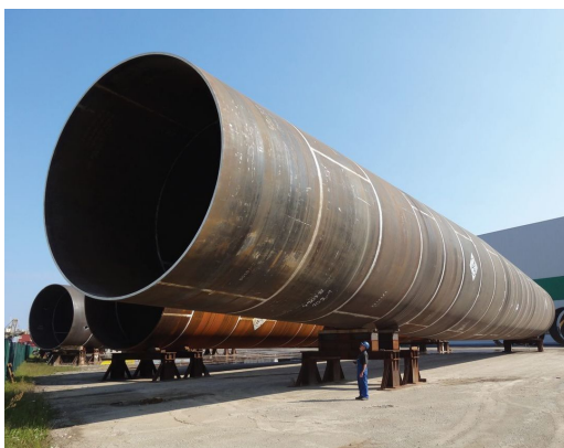
Figure 1.1: Monopile before installation [1]
