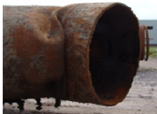
Figure 1.2: Buckling in a monopile [2]
