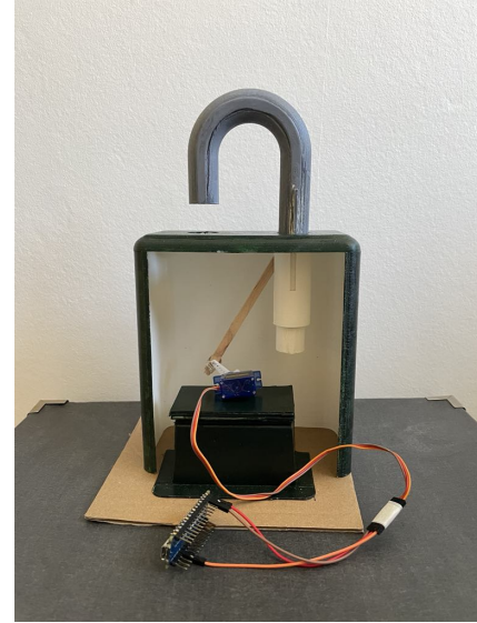
Fig. 2: Setup of Padlock: 1) Shackle, 2) Peg to connect motor and shackle, 3) Arm of servo motor, 4) Servo motor, 5) Arduino Nano 33 BLE board
