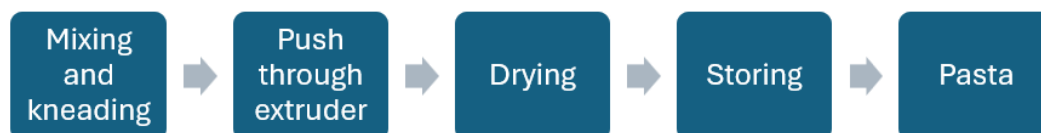
Figure 11 Wheat pasta-making process adapted from (Chen, 2024)
