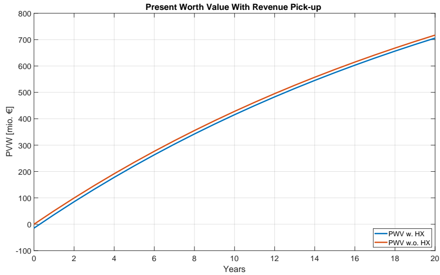
Figure 5.1: Present Worth Value with revenue pick-up. The electricity price is € 75/MWh and the interest rate is 8%
