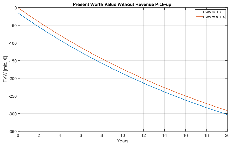
Figure 5.2: Present Worth Value without revenue pick-up. The electricity price is €75/MWh and the interest rate is 8%
