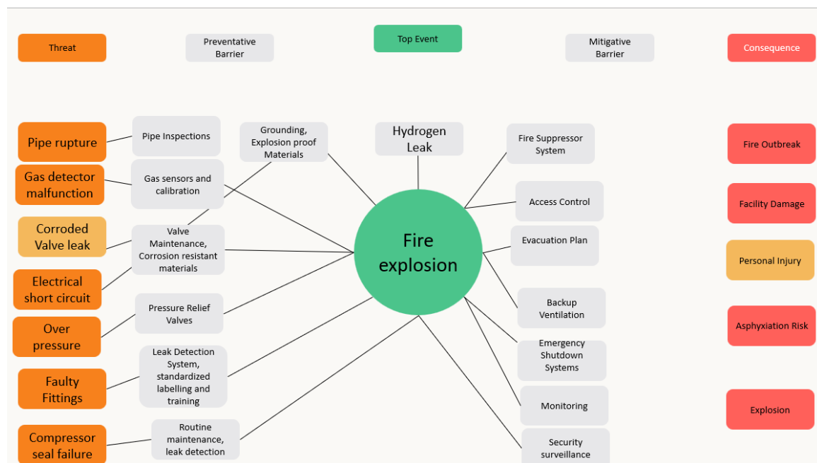
Figure 9: Bowtie Analysis of a potential hydrogen leak leading to a fire explosion
