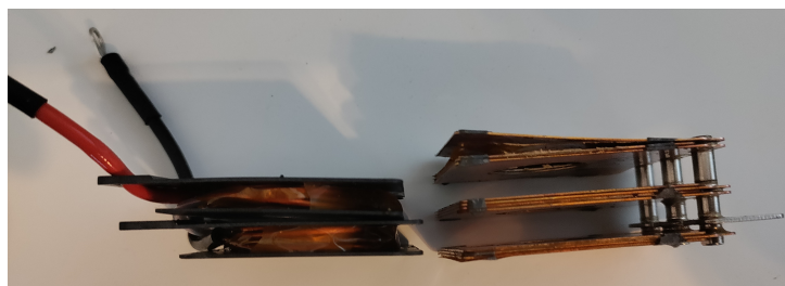
Figure 2.6 PREMO Semi-Planar windings split up into two with wire winding on the left and planar on the right.
