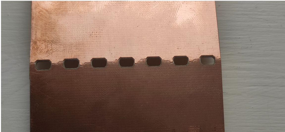
Figure G.10 Bottom side of the mechanical test specimen "Eco4" after the three-point-bending test.
