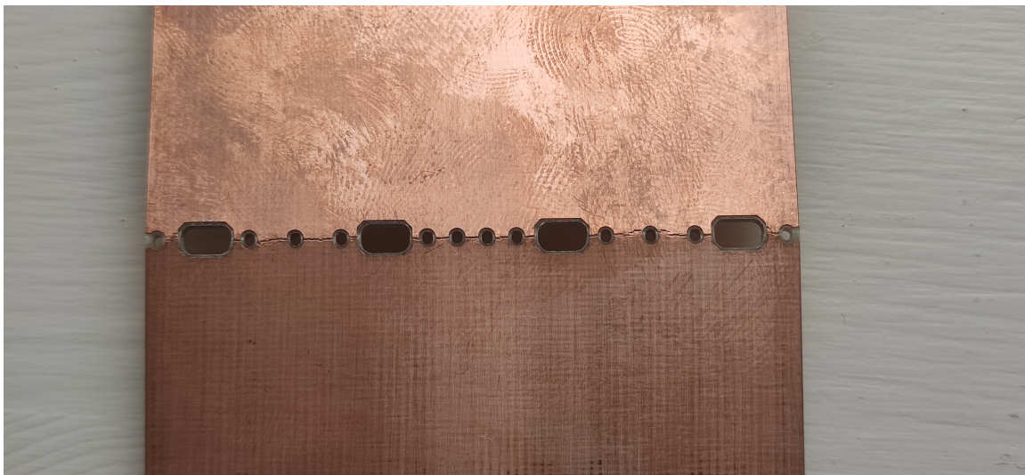
Figure G.14 Bottom side of the mechanical test specimen "EcoSH" after the three-point-bending test.
