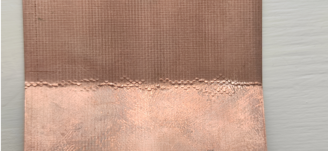
Figure G.1 Top side of the mechanical test specimen "Conv" after the three-point-bending test.
