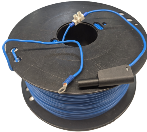
Figure 4.14 Ramping inductor with air core.
