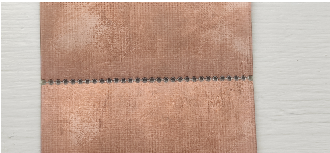
Figure G.5 Top side of the mechanical test specimen "Eco2" after the three-point-bending test.
