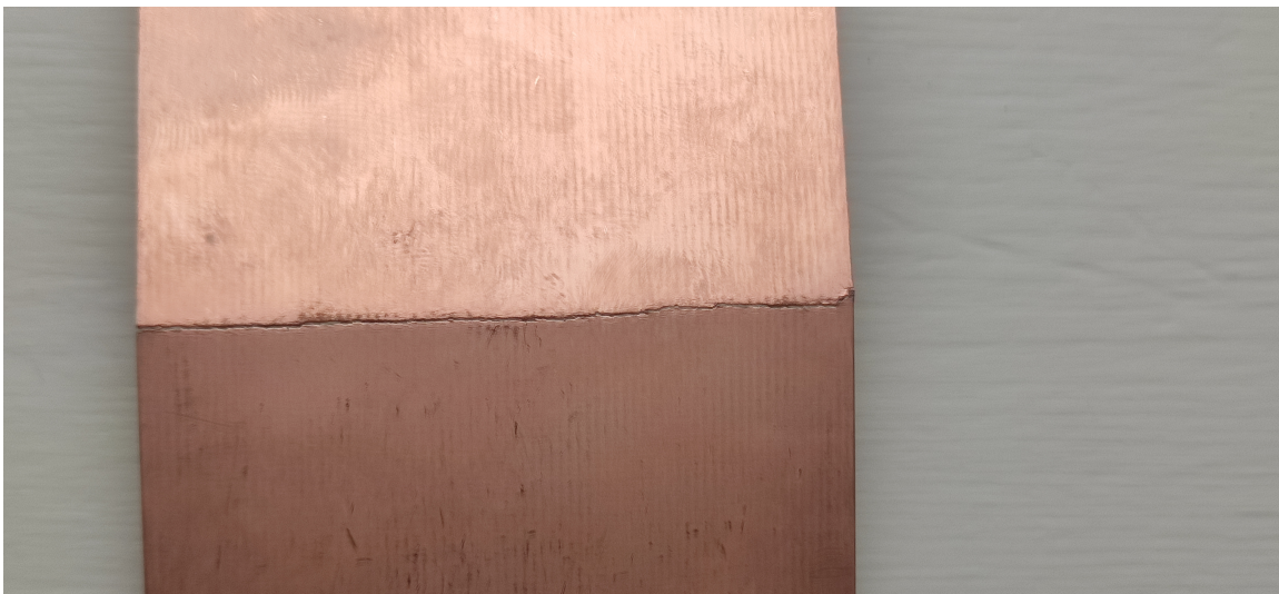
Figure G.2 Bottom side of the mechanical test specimen "Conv" after the three-point-bending test.
