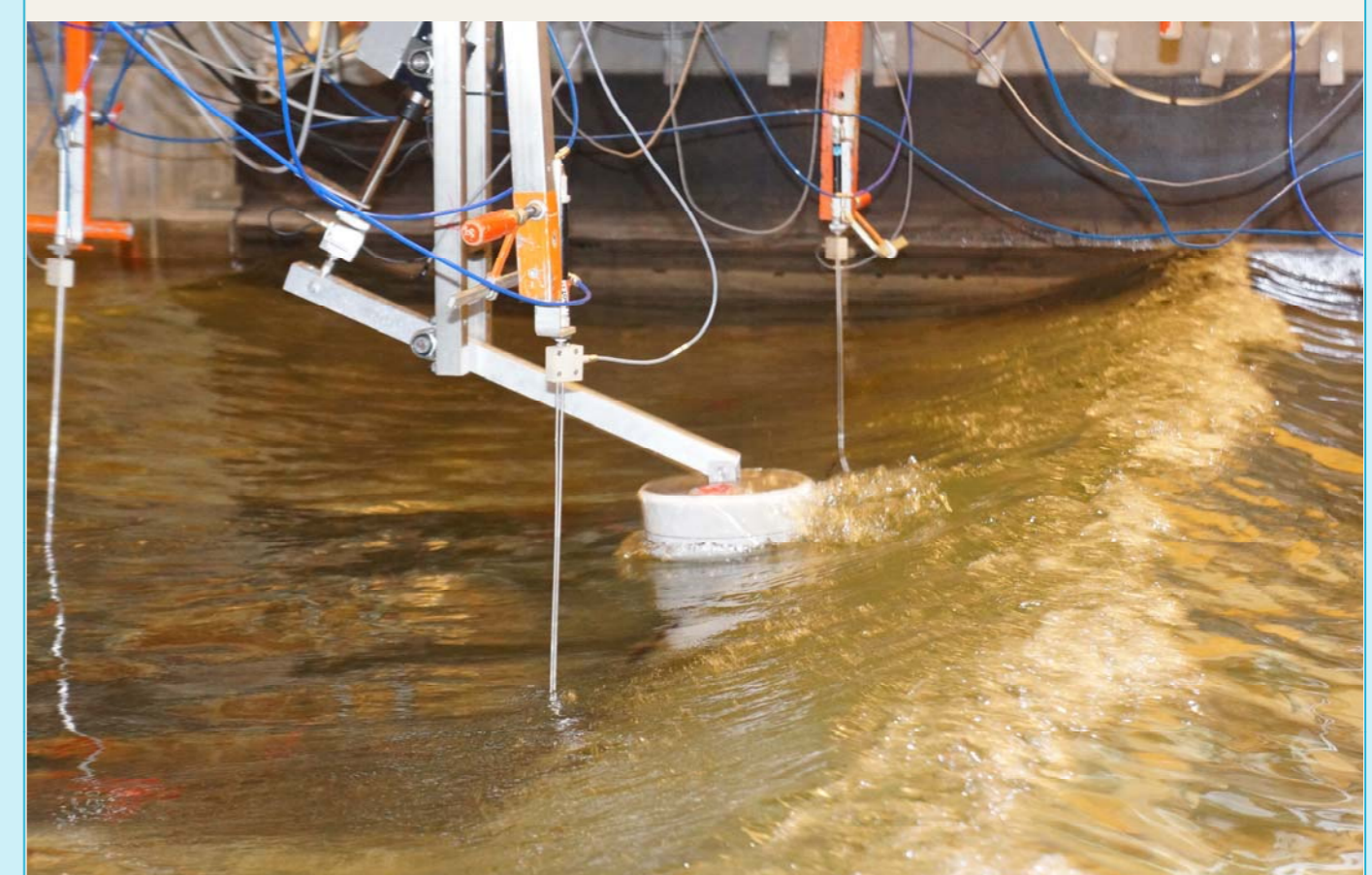
Figure 7: Glass fiber float on pivot arm in wave basin.
