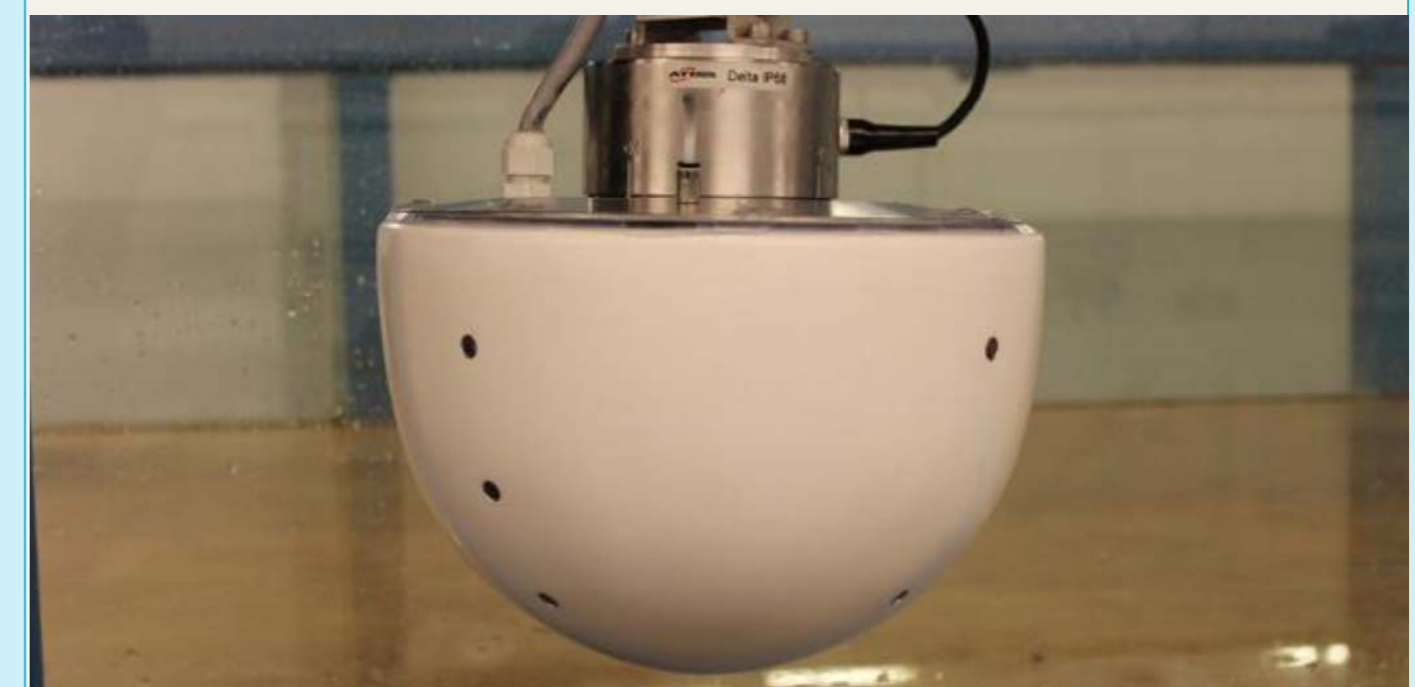
Figure 6: Model used in experiments equipped with pressure sensors and a 6-axis F/T-transducer.
