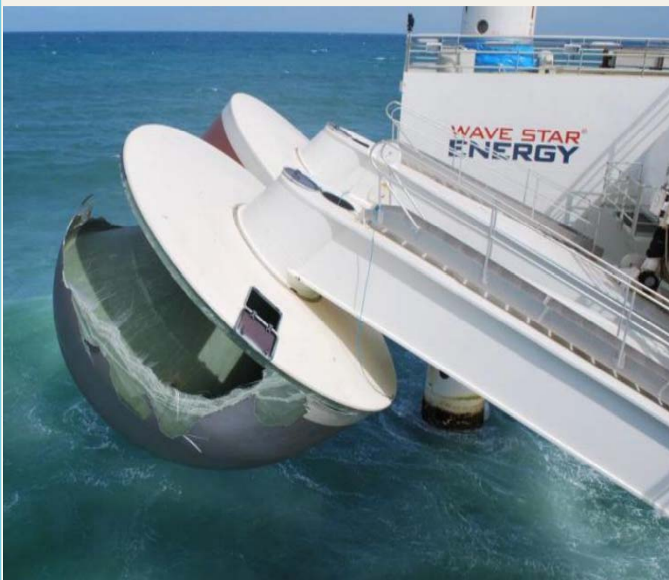
Figure 2: Fractured glass fiber prototype float.
