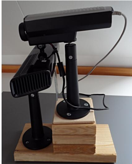
**Figure 5.1:** Hardware platform containing the AXIS Q1922 and the Microsoft Kinect for XBOX.
