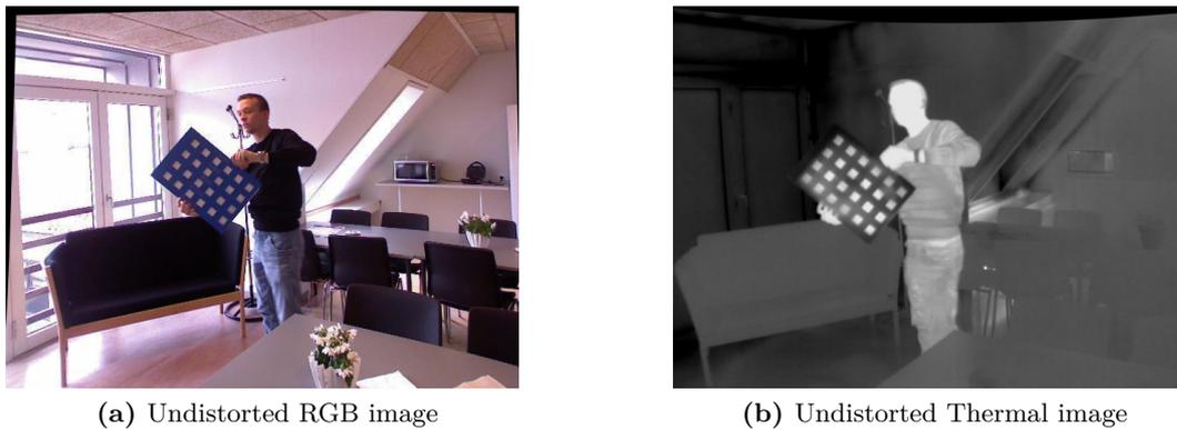
**Figure 6.9:** Undistorted calibration images. The lens distortion is removed from both cameras and straight lines appear straight in both images.
