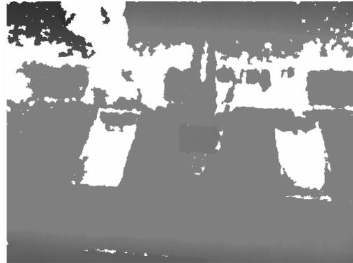
(b) Depth image of object at 4 metres from the sensor. The depth value returned from the Kinect sensor is 3074 mm.
