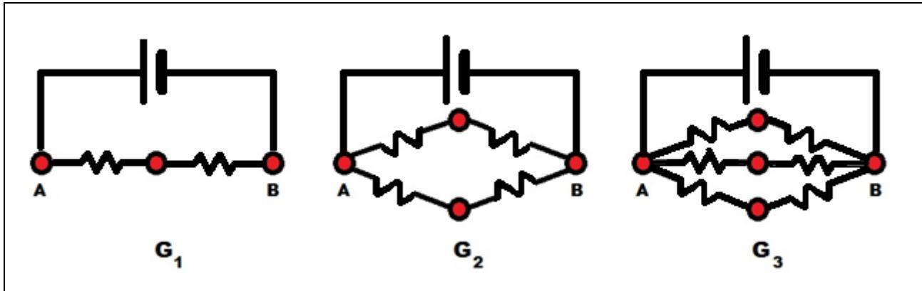
**Figure 3: The three graphs of Figure 2 with resistors introduced on each edge, while a battery is linked between the a,b-pair of vertices. (Klein & Randic, 1993)**
