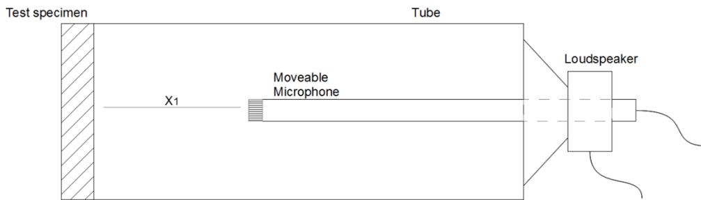
**Figure 5.17** – Illustration of the standing wave method in tube measurement setup. The microphone is moveable to detect pressure minima and maxima at distance  $X1$ .
