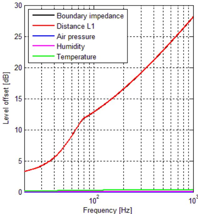
**Figure 5.15** – Possible level offset in dB caused by the characteristics within their normal range. The boundary impedance, black line, is hidden behind the distance L1, red line.
