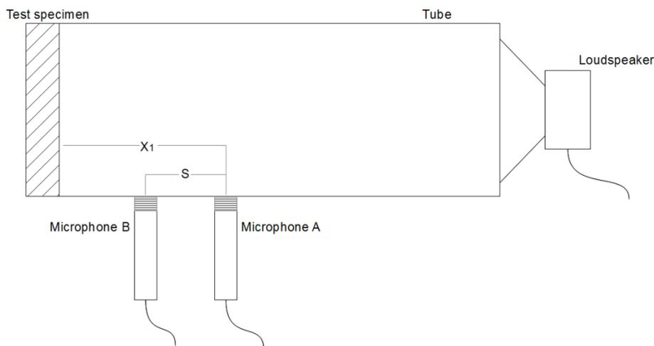
**Figure 5.18** – Illustration of the transfer function method in tube measurement setup.
