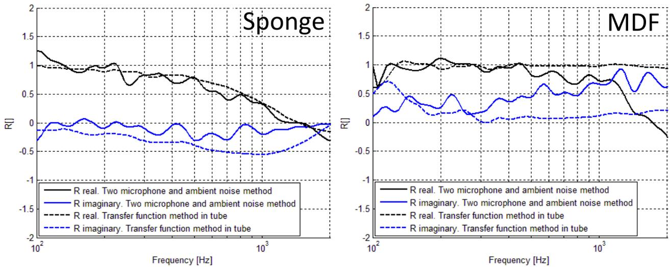
**Figure 6.17** – Reflection factors measured using the two microphones and ambient noise method and the transfer function method in tube. Real and imaginary values.
