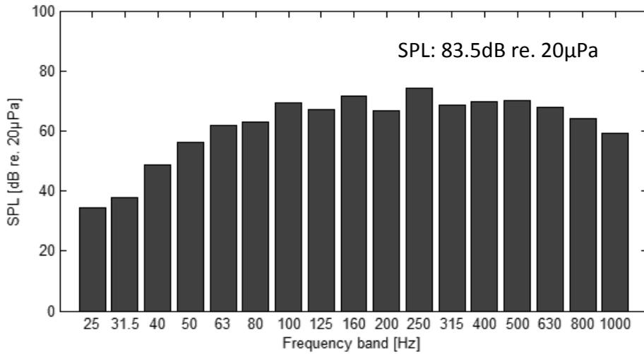
Figure 6.15 – SPL level in 1/3 octave band for pulsed pink noise with increased sound pressure level. Noise no. 4.
