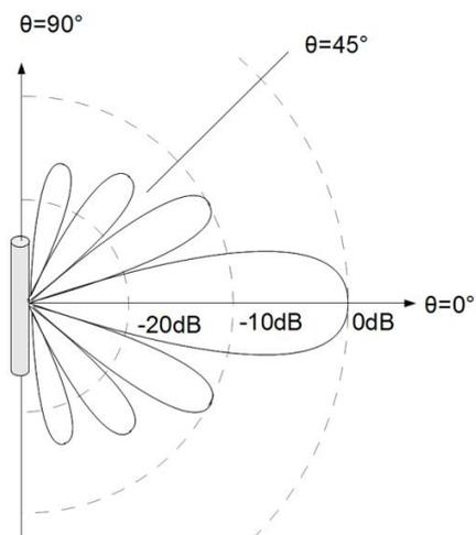
**Figure 5.3** – Illustration of a beam pattern for a continuous line source radiation sound at a certain frequency. Depends on line source length and frequency, the beam pattern will look different.
