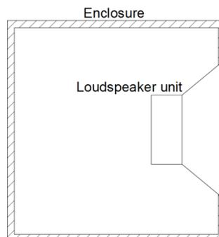
**Figure 5.1** – Illustration of the loudspeaker consisting of a dynamic loudspeaker unit and a closed enclosure.
