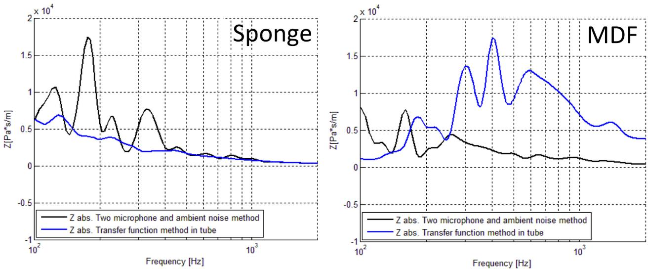
Figure 6.20 – Impedances measured using the two microphones and ambient noise method and the transfer function method in tube. Absolute values.
