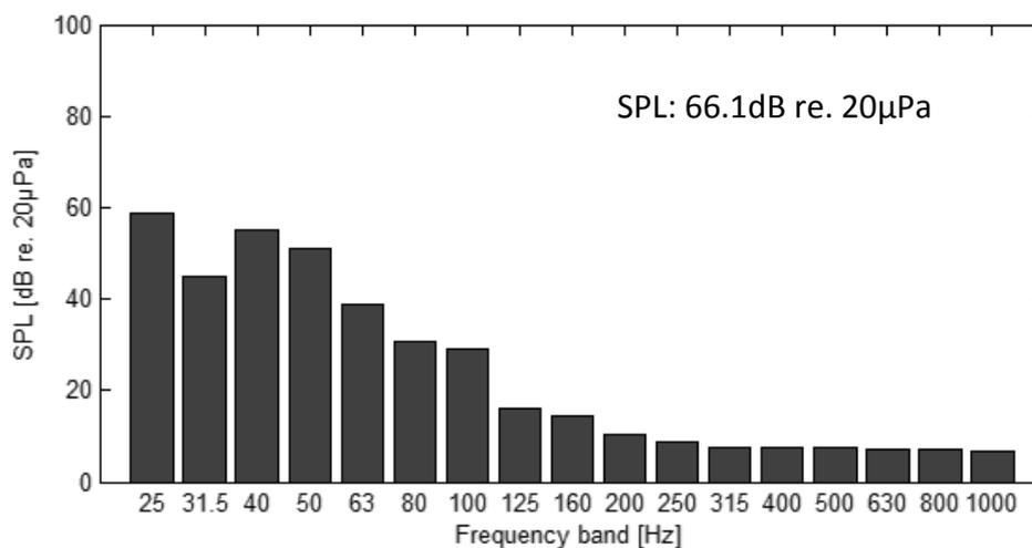
**Figure 6.12** – SPL level in 1/3 octave band for existing ambient noise in the standard stereo listening room. Noise no. 1.
