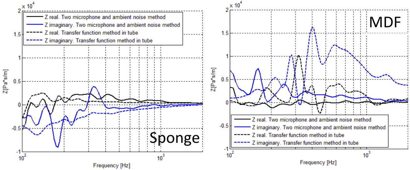
Figure 6.19 – Impedances measured using the two microphones and ambient noise method and the transfer function method in tube. Real and imaginary values
