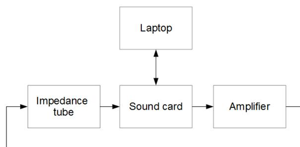
**Figure 6.8** - Setup and connections between equipment for the transfer function method in tube.
