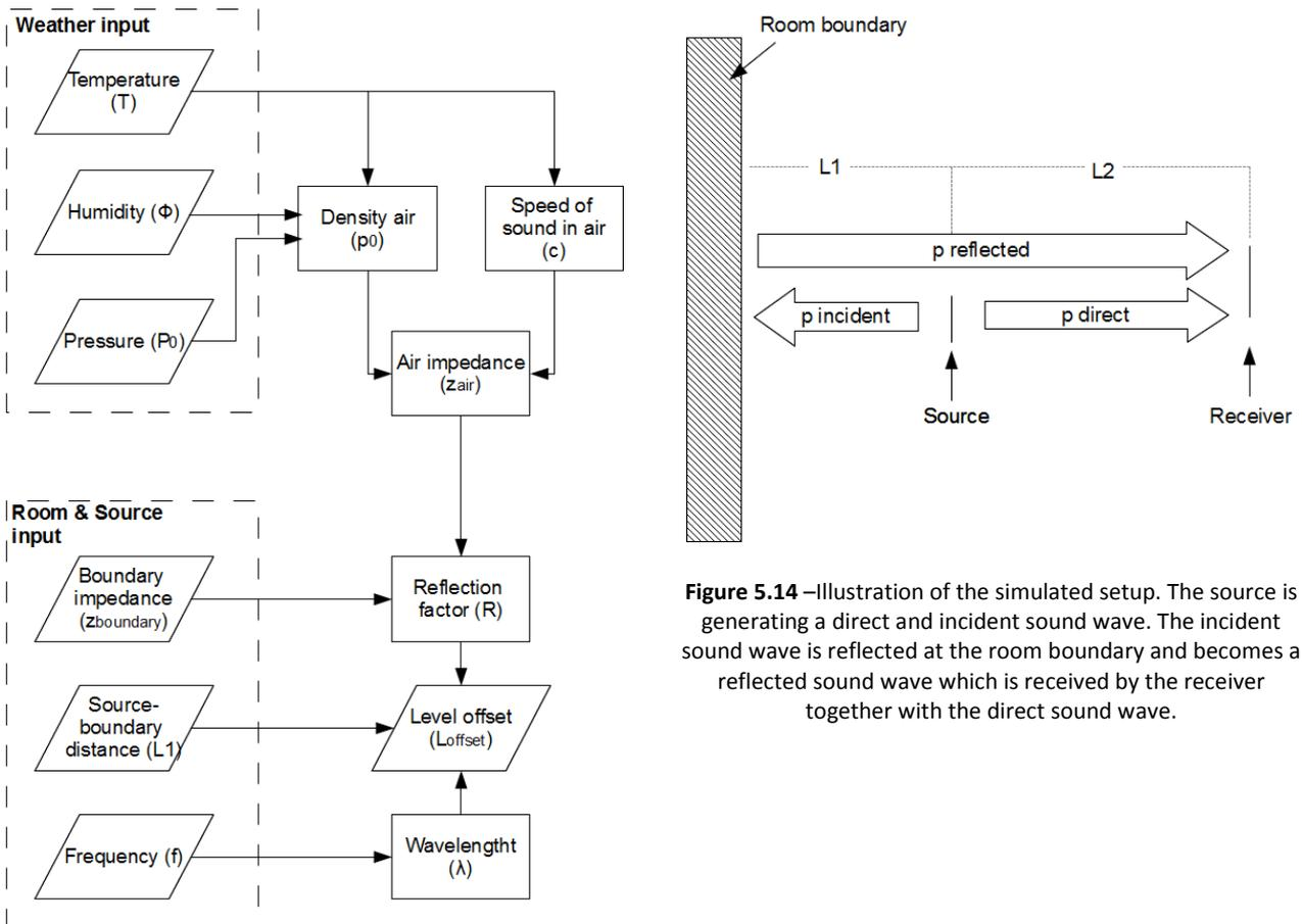
**Figure 5.13** – Flowchart of the level offset calculations used in the simulation. The inputs are varied while change of level offset is observed.
