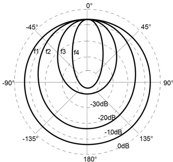
**Figure 5.4** – Polar plot Illustration of a general monopole loudspeaker which may be a single loudspeaker unit mounted in a closed enclosure as in **Figure 5.1**.  $f_1$  is the lowest frequency and  $f_4$  is the highest. The higher frequency the narrower the radiation pattern.
