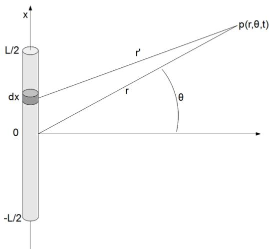
**Figure 5.2** – Illustration of a continuous line source with length  $L$  and radius  $a$ . The pressure,  $p$ , in far field is calculated using the distances  $r$  and  $r'$ , the angle,  $\theta$ , and simple sources along the line source with length  $dx$ .
