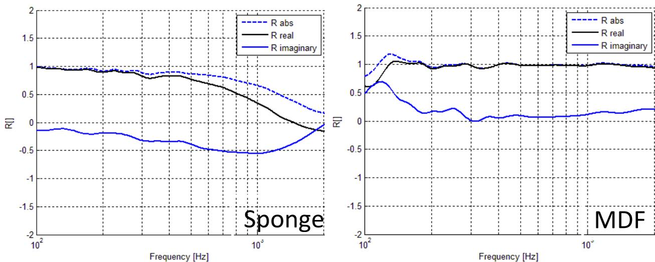
**Figure 6.9** – Measured reflection factors for the sponge mat and MDF board using transfer function method in tube.
