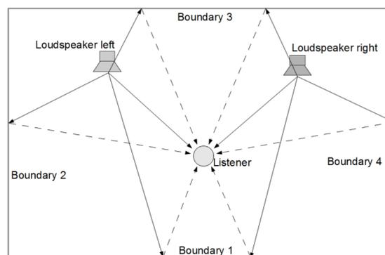
**Figure 5.7** – Illustration of first order reflections in a rectangular room with a stereo setup. The solid lines are the direct sound waves and the dashed lines are reflected sound waves. 1. order reflections from left loudspeaker on boundary 4 and from right loudspeaker on boundary 2 will also exist but is leaved out for the sake of simplification.
