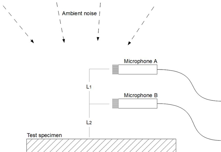
Figure 8.8 – Microphones and test specimen setup.
