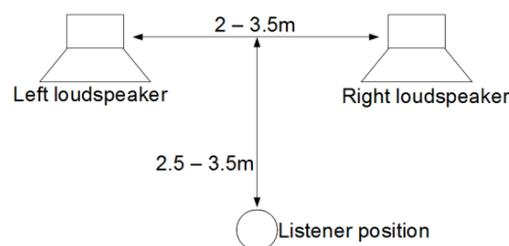
**Figure 5.6** – The stereo setup and distances proposed by [IEC 60268-13].
