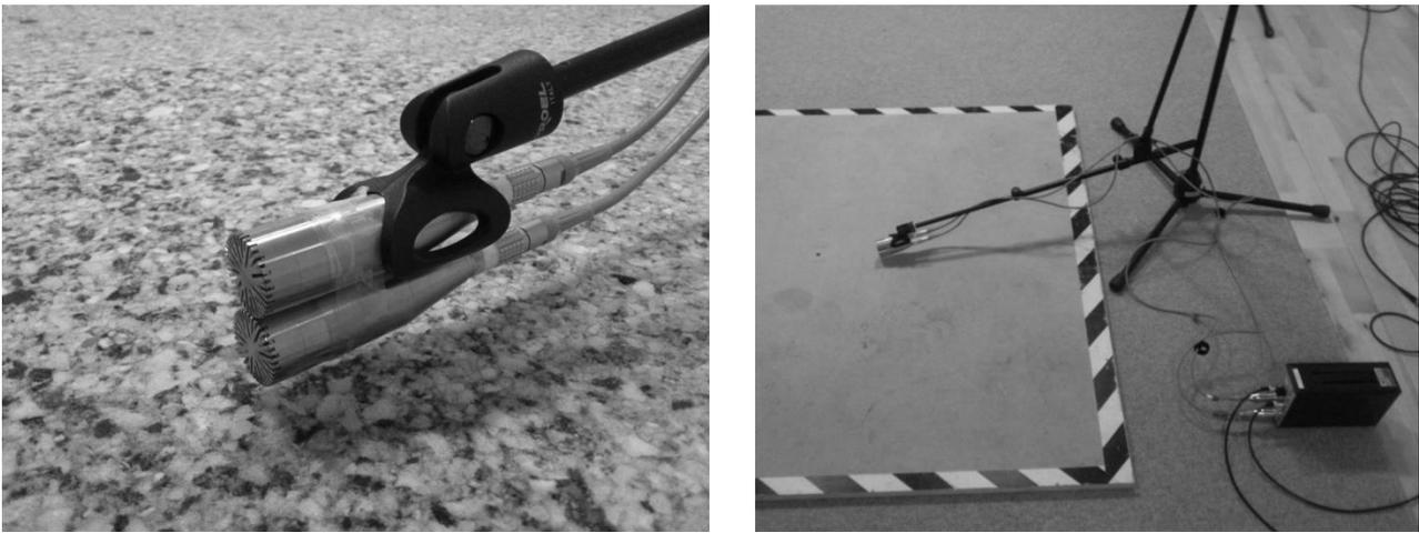
**Figure 6.3** – Picture of the setup in the standard stereo listening room. Left: close up picture of the two microphones and the sponge mat. Right: picture of the microphone stand, phantom power supply, microphones and MDF board.
