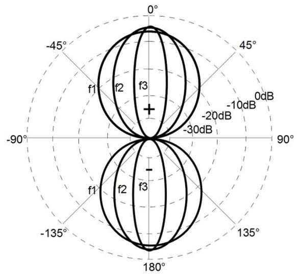
**Figure 5.5** - Polar plot Illustration of a general bipolar loudspeaker which radiates as a figure of 8.  $f_1$  is the lowest frequency and  $f_3$  is the highest. The higher frequency the narrower the radiation pattern.
