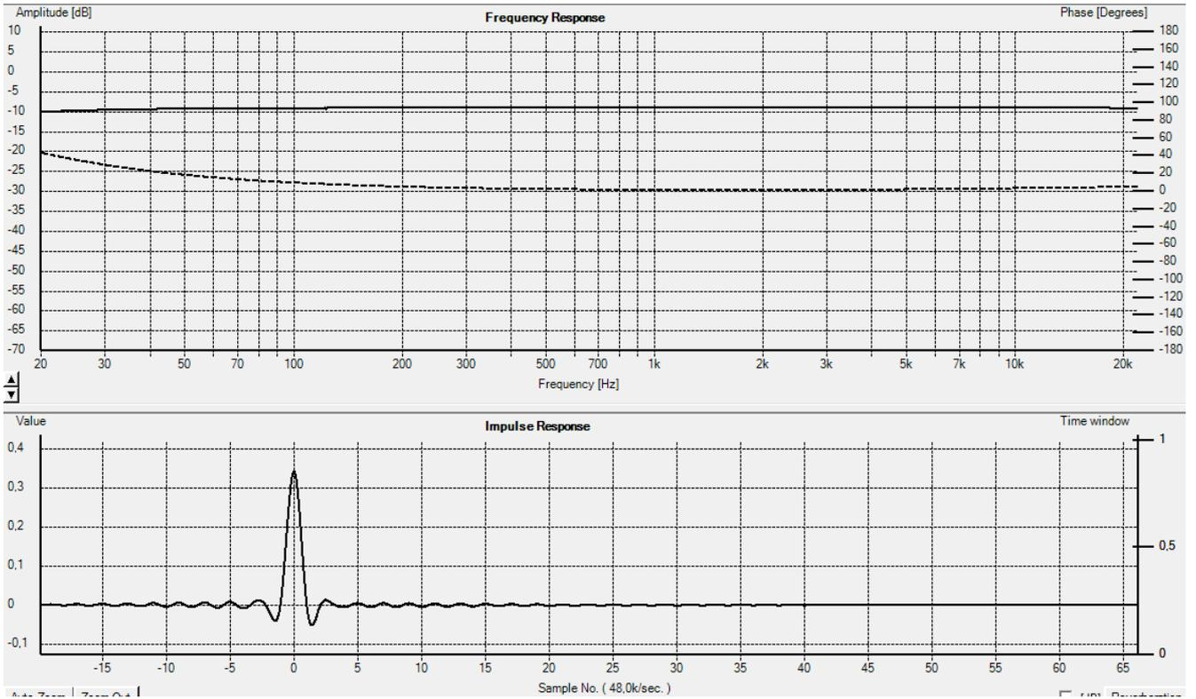
**Figure 8.3** – The impulse, frequency and phase response for soundcard input channel 2. The frequency response is the solid line and the phase response is the dashed line.
