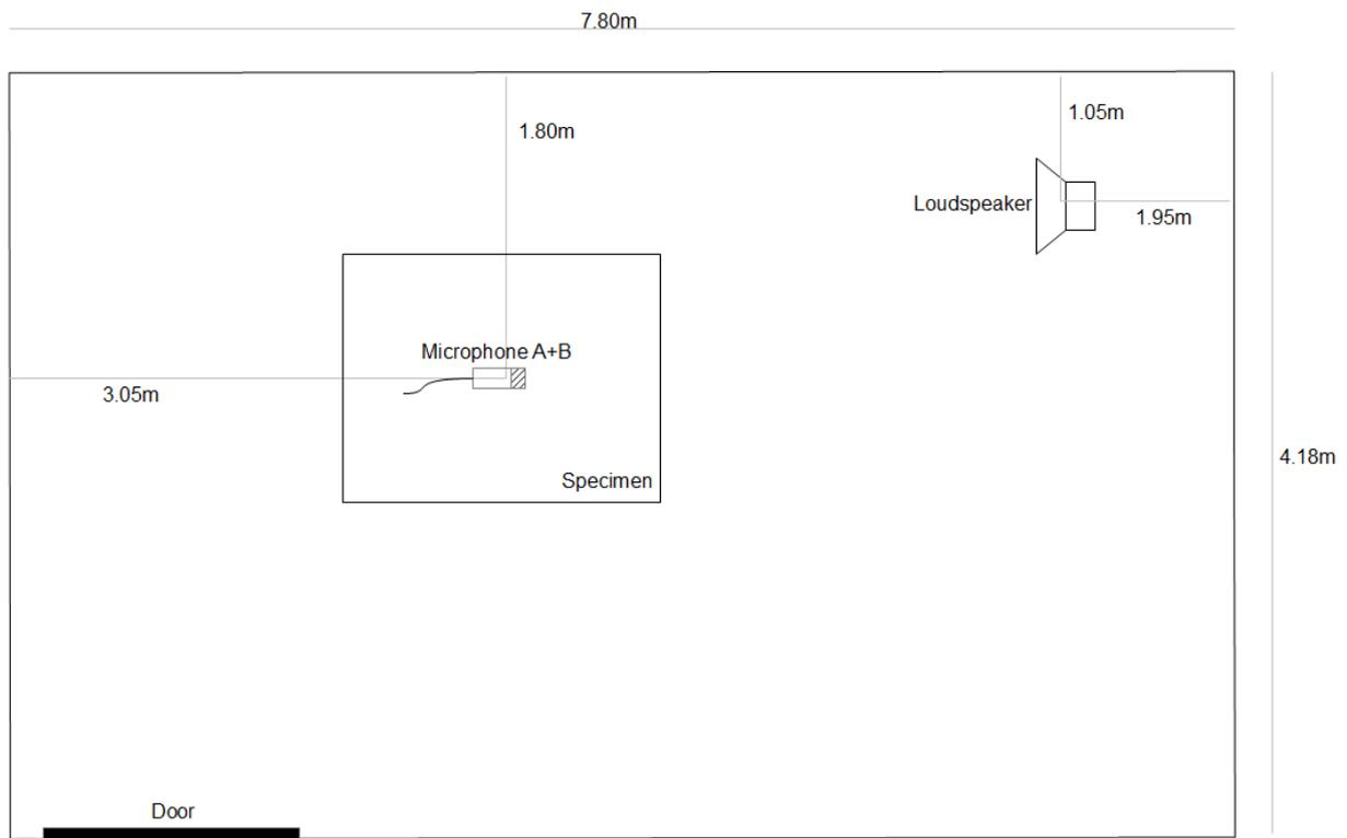
Figure 8.10 – Equipment and test specimen positions in the standard stereo listening room.
