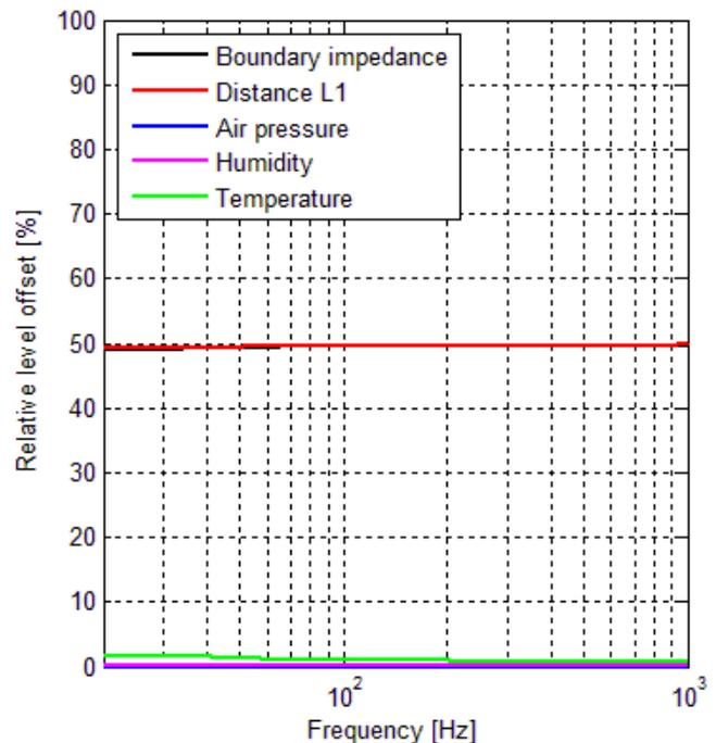
**Figure 5.16** – Relative level offset in % caused by the characteristics within their normal range. The boundary impedance, black line, is hidden behind the distance L1, red line.
