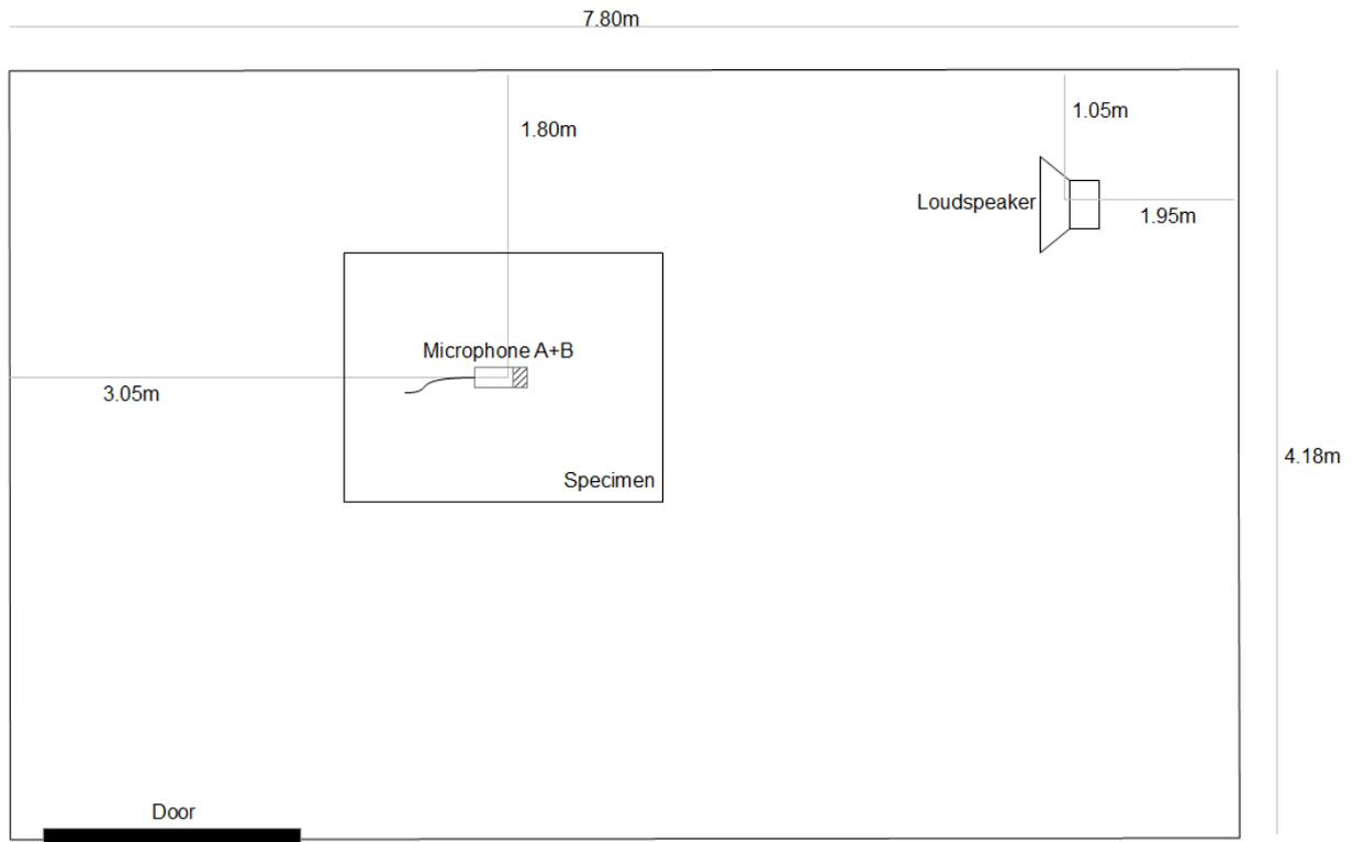
Figure 8.7 – Equipment and test specimen positions in the standard stereo listening room.
