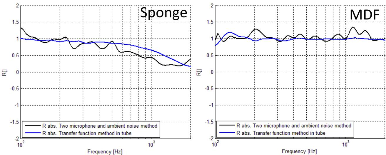
**Figure 6.18** – Reflection factors measured using the two microphones and ambient noise method and the transfer function method in tube. absolute values.
