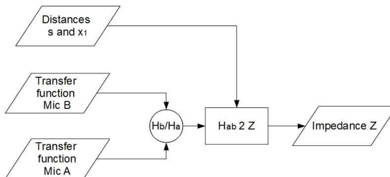
**Figure 6.7** – Signal processing flowchart for the transfer function method in tube. The inputs are the distances and transfer functions for microphone A and B and the output is the impedance. The Hab2Z block calculates the impedance with use of the transfer function between microphone A and B and the distances. Hab2Z is based on equation (5.48) and (5.49) section 5.6.1.3.
