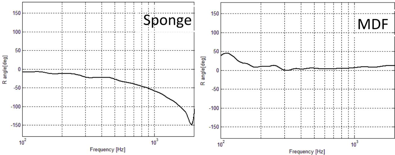
Figure 6.10 – Measured reflection factor phases for the sponge mat and MDF board using transfer function method in tube.
