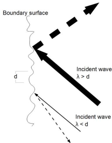
**Figure 5.8** – Illustration of how sound waves, with short and long wavelength compared to the boundary surface, will be reflected. The solid lines are incident waves and the dashed lines are reflected waves.
