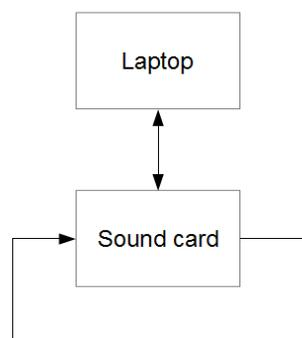
Figure 8.1 – Flowchart of the measurement setup. The soundcard outputs are looped back to the inputs.
