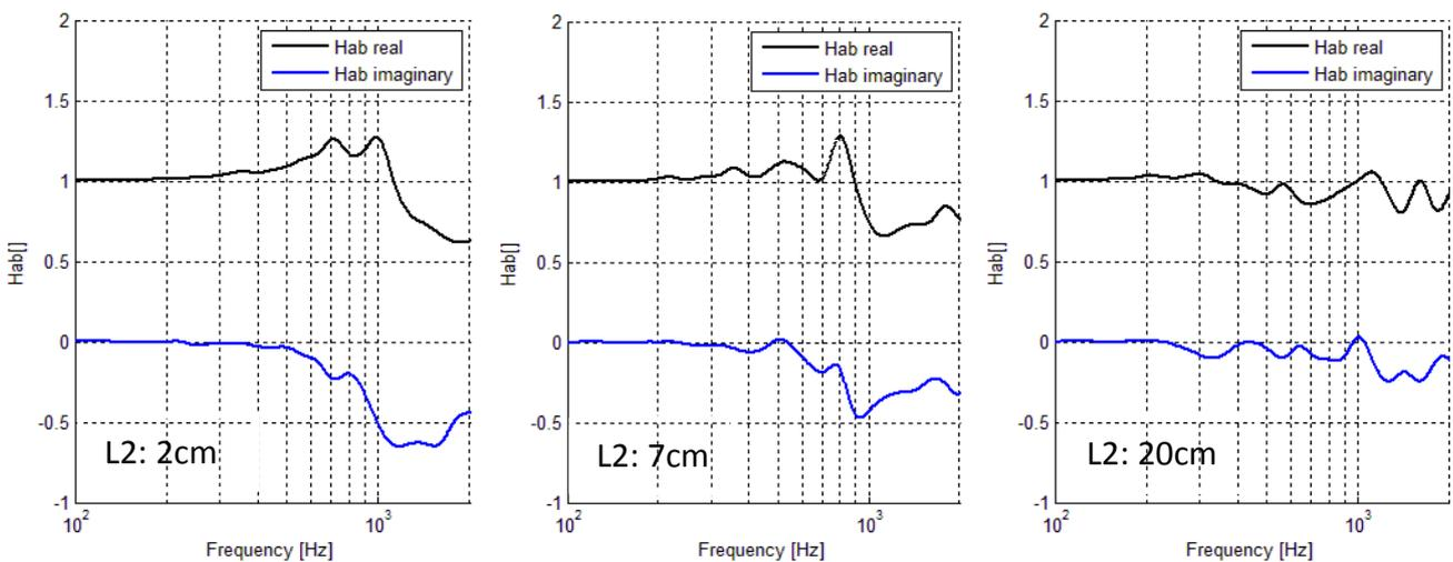
Figure 6.16 – The measured transfer function between microphone A and B for different distances between the microphones and test specimen. From left to right the distances are respectively 2, 7 and 20 cm and the transfer function becomes closer to 1 for the real part and 0 for the imaginary part. The sponge mat is used as the test specimen in all 3 cases.
