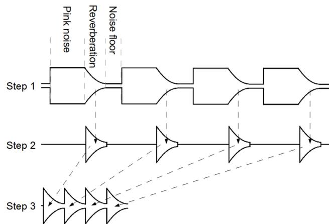
**Figure 6.5** – Signal processing of the pulsed noise signal, noise no. 4 or 5. Step 1 is the raw signal with pulsed pink noise, reverberation tails and noise floor. Step 2 is the result when windows are applied around the reverberation tails to remove the pink noise and noise floor. In step 3 the zeroes between the reverberation tails are removed.
