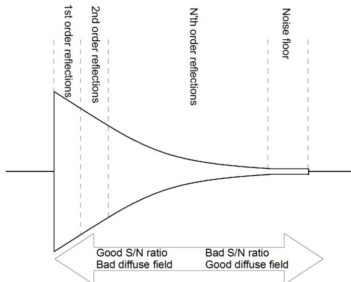
**Figure 6.6** – Illustration of a single reverberation event. The first part is dominated by the 1<sup>st</sup> order reflections, 2<sup>nd</sup> order reflections and so forth. The longer the time period after the reverberation event start, the higher order reflections will dominate which lead to better diffuse field.
