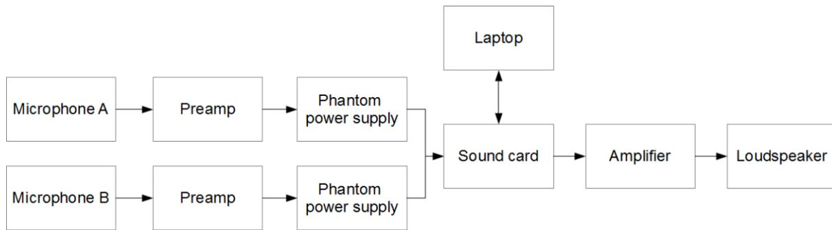
**Figure 6.2** – Setup and connections between equipment for the two microphones and ambient noise method.
