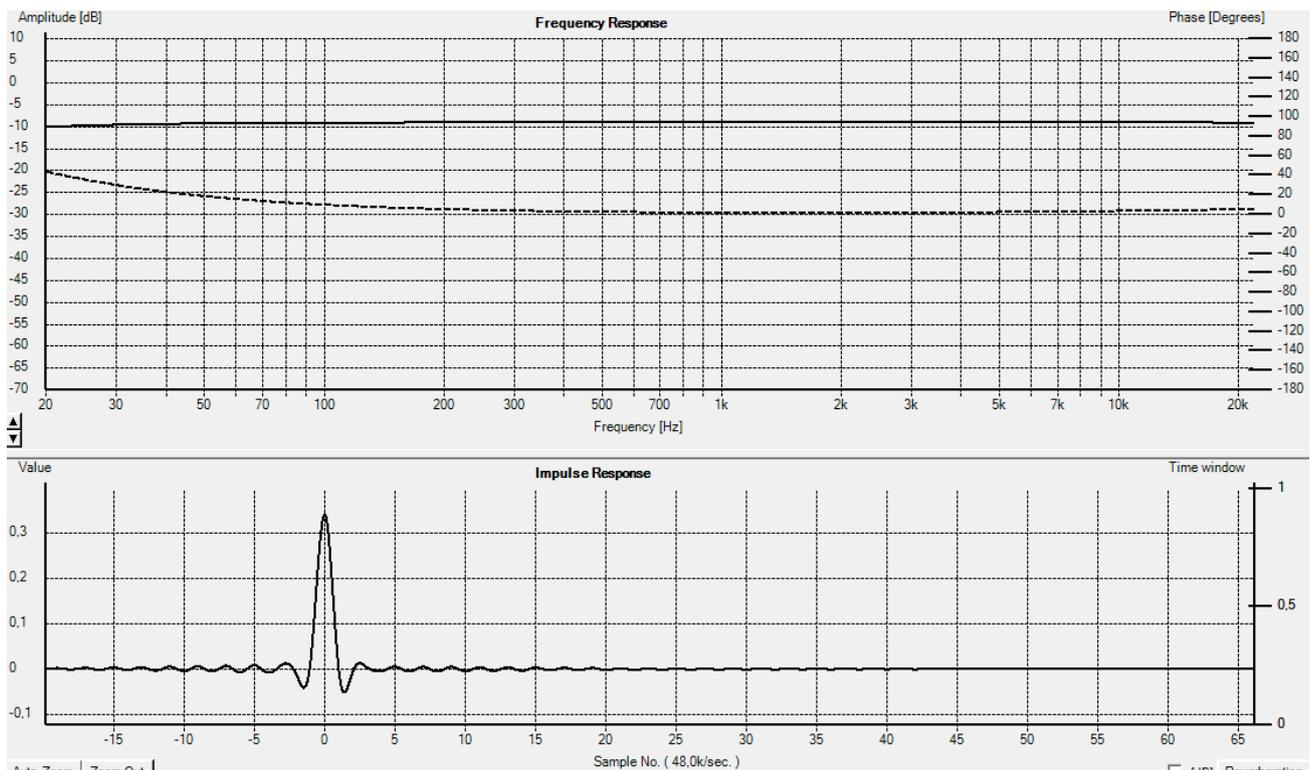
**Figure 8.2** – The impulse, frequency and phase response for soundcard input channel 1. The frequency response is the solid line and the phase response is the dashed line.
