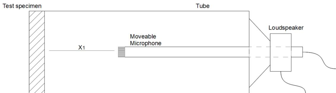
**Figure 8.5** – Setup in the impedance tube.
