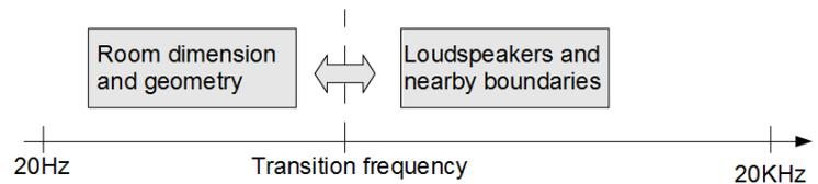
**Figure 5.9** – Illustration of which factors that dominate the behavior of sound, radiated from loudspeakers, in a room, depends on frequency.
