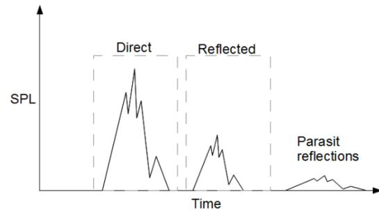
Figure 5.20 – Illustrated impulse response measured with the transfer function method with applied time windows on the direct and reflected sound.
