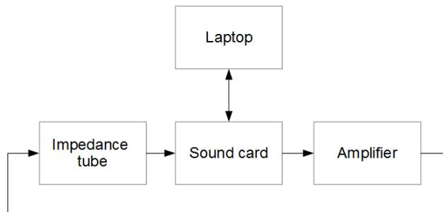
**Figure 8.4** – Setup and connections between equipment.
