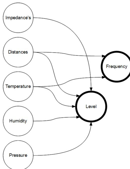
**Figure 5.12** – Illustration showing which characteristics that influences the frequency and level using the theory from section 5.2.
