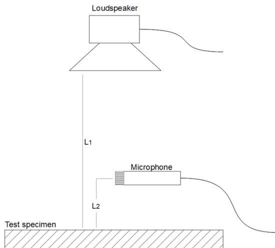
Figure 5.19 – Illustration of the in situ transfer function method measurement setup.
