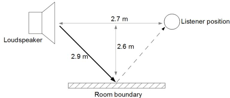
**Figure 5.11** – Side view illustration of critical distances between loudspeakers and boundaries following the stereo setup in [IEC 60268-13]. It is assumed that the listener and loudspeaker height are equal. A longer distance between the loudspeaker and listener position will increase the critical distances.
