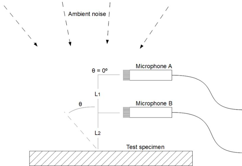
**Figure 5.21** – Illustration of the two microphones and ambient noise method measurement setup.
