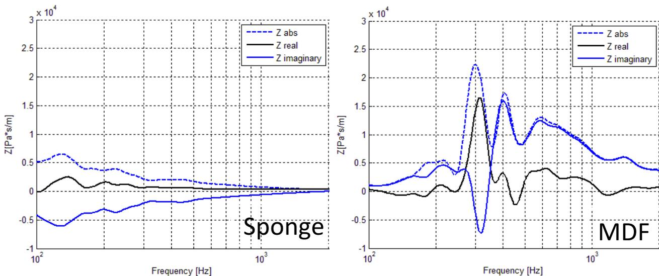
Figure 6.11 – Measured impedances for the sponge mat and MDF board using transfer function method in tube.
