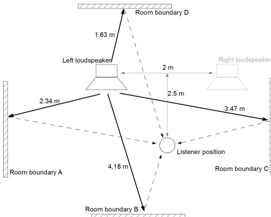
**Figure 5.10** – Top view illustration of critical distances between left loudspeakers and boundaries following the stereo setup in [IEC 60268-13]. Boundaries within the distances will contribute to timbre changes. A longer distance between the loudspeaker and listener position will increase the critical distances.
