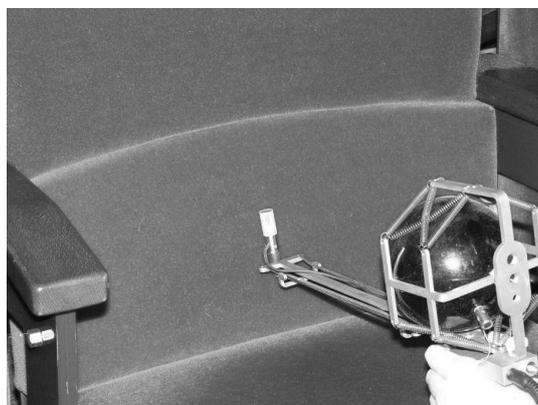
**Figure 5.23** – Picture of a handheld measurement setup with the PU probe, measuring the impedance of a chair backrest. The black sphere contains a small loudspeaker used as sound source and the small cylinder, close to the backrest, is the PU probe [Microflown].
