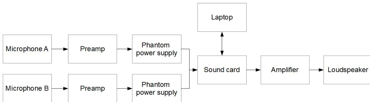
Figure 8.6 – Setup and connections between equipment.
