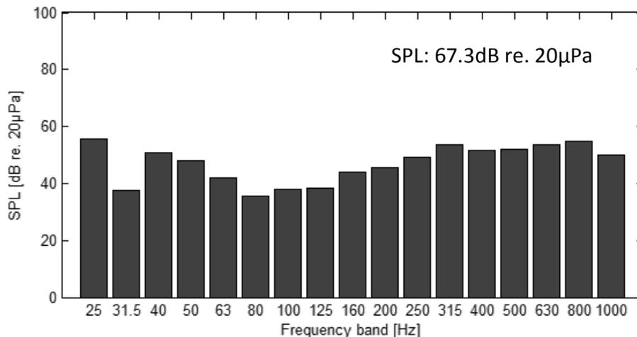
**Figure 6.14** – SPL level in 1/3 octave band for pink noise and pulsed pink noise highpass filtered at 130Hz. Noise no. 3 and 5.
