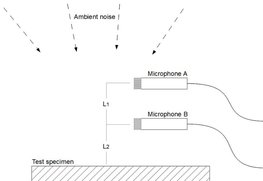
Figure 8.11 – Microphones and test specimen setup.
