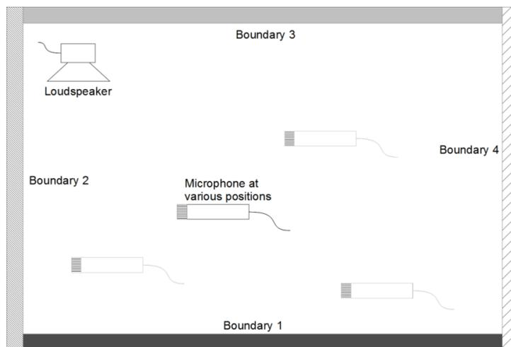
**Figure 5.22** – Illustration of the inverse method measurement setup.
