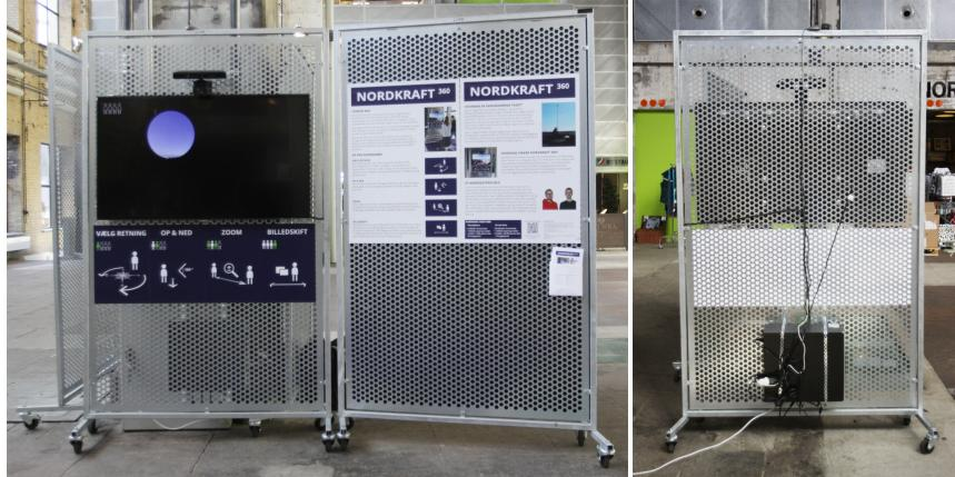
Fig. 1. (Left) An image of Nordkraft 360, showing the four interaction illustrations beneath the display, along with the interaction and information poster hanging to the right of the system. (Right) The back of the system is shown, with the computer and cables attached to the metal stand.
