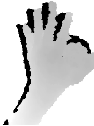
Figure 6.1. When relying purely on depth information it can be difficult to distinguish between the cup and the hand when they are close to each other in all three dimensions. In this picture the cup is located between the thumb and the index finger.
