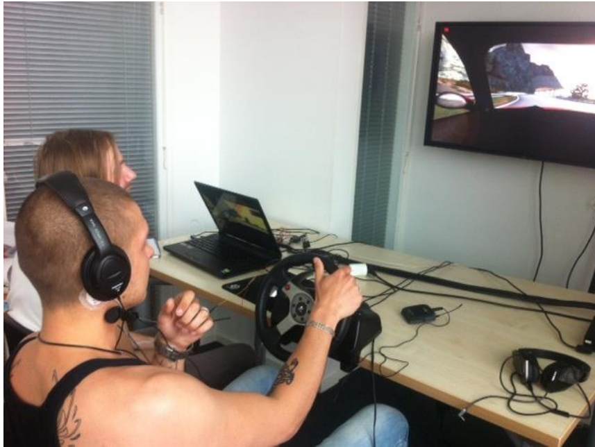
Figure 20. Test subject from first condition group receiving GVS while driving and having to verbally express arithmetic task results
