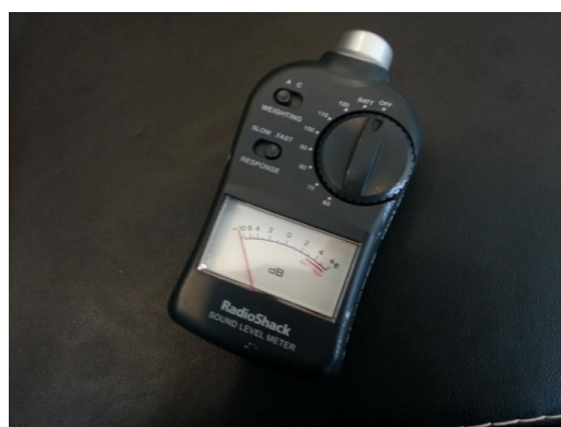
Figure 7, shows the sound pressure meter used to calibrate sound pressure before the test.
